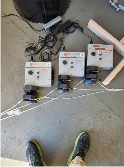
Photograph 3. Low-flow peristaltic pumps.
