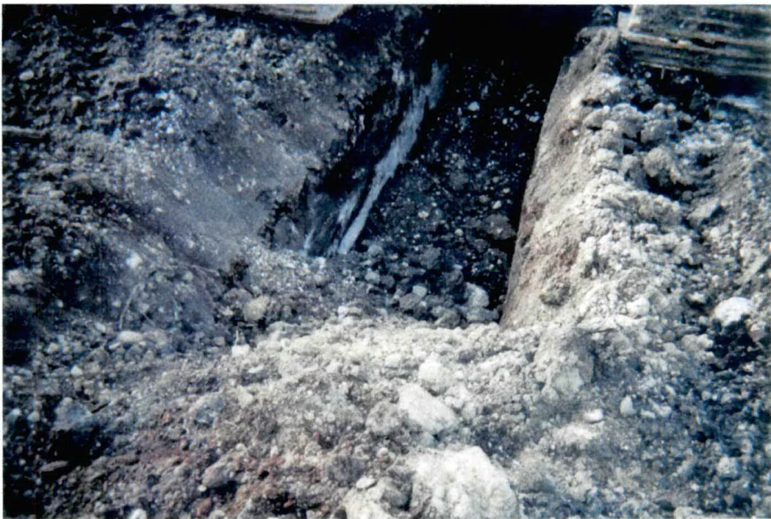
Photograph #2 – View of TP-1 showing CKD material.
