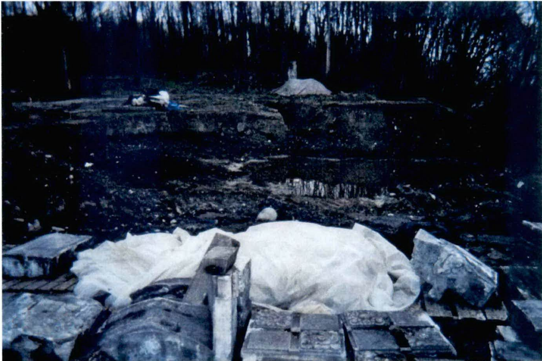
Photograph #2 – View of battery casing material found on the north side of the former CKD excavation pit.
