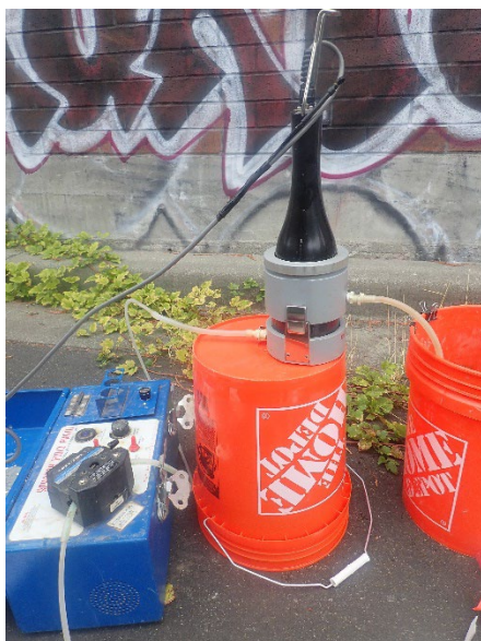
View of purging in progress (note use of a flow cell for parameter monitoring).
