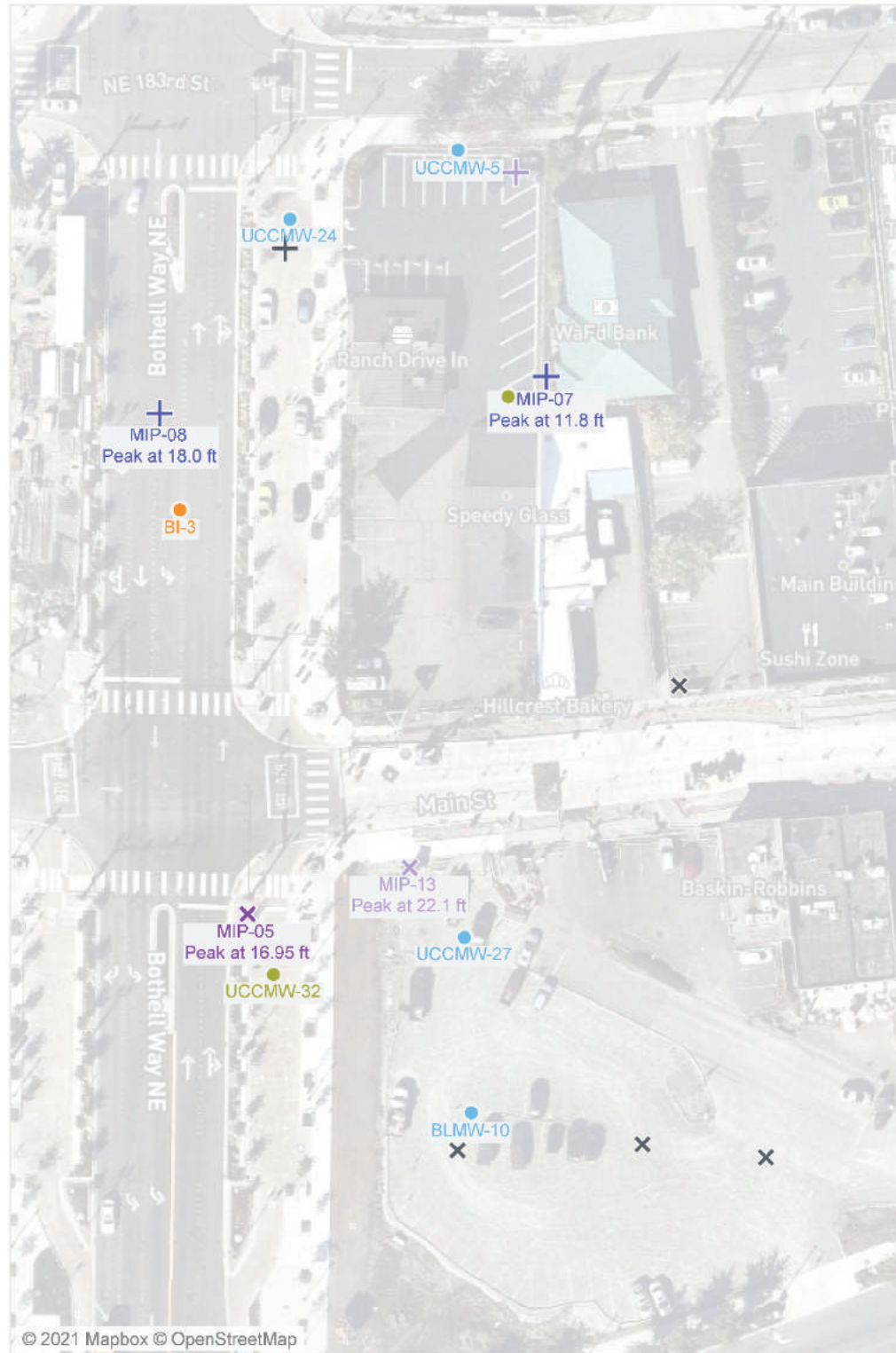
Collocated Shallow Aquifer Zone Groundwater Results and MIP Responses MIP results with maximum response in shallow zone are labeled.
