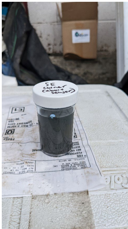
Photograph 28. Sudan IV field screening results from soil collected above storm sewer at 6.5 feet bgs. Lack of meniscus indicates total petroleum hydrocarbon concentrations less than residual saturation limits.
