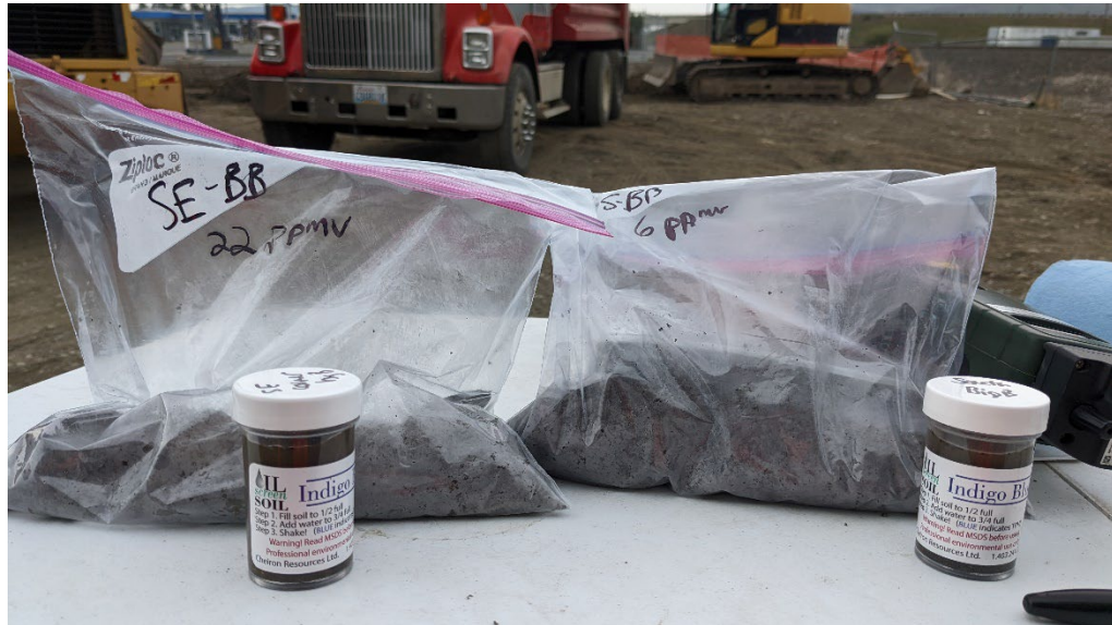
Photograph 25. Sudan IV field screening results from 2021 backfill on the southeast corner of the Big B property adjacent to excavated LNAPL collection trench. No visible meniscus or styrene ball discoloration, indicating total petroleum hydrocarbon concentrations less than residual saturation limits.
