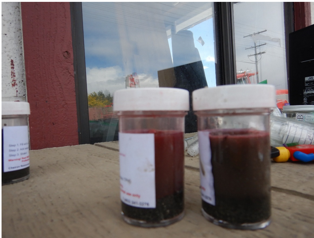
Photograph 10. Sudan IV results for SIDE-09 and SIDE-10 areas before overexcavation at SIDE-09.
