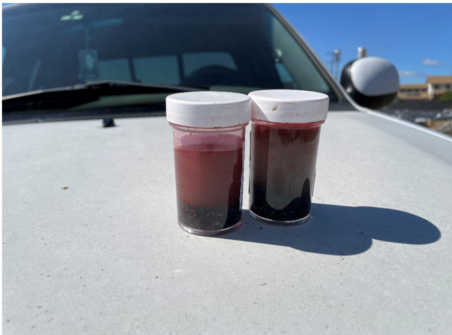
Photograph 14. Sudan IV results for BASE-10 at 7 and 8 feet below ground surface (bgs). Results of field screening indicated that deeper excavation was required.
