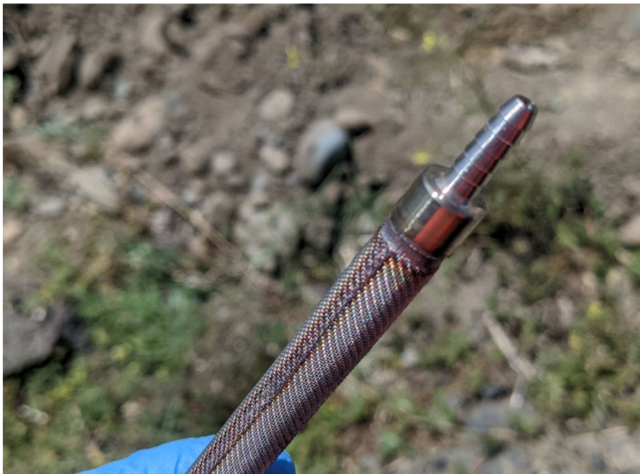
Photograph 56. Three-inch-long, stainless steel soil vapor screen. The screen was attached to tubing and installed at 3 feet bgs.
