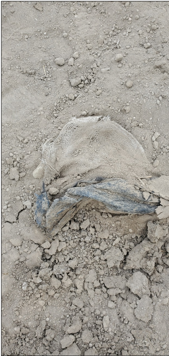
17. 2022: Damaged geosynthetic liner.
