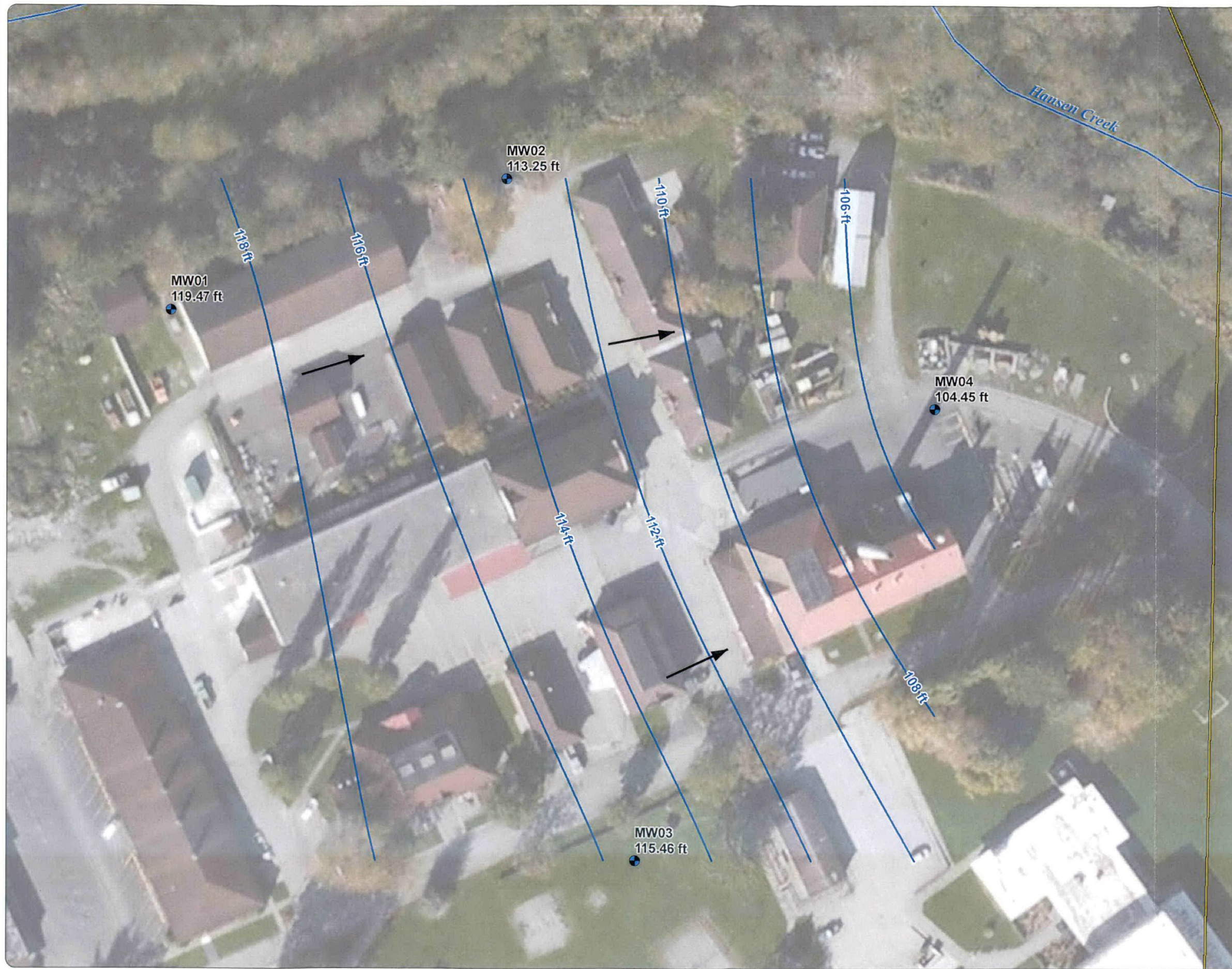
Figure 5 Groundwater Elevation Contours Northern State Hospital Property Port of Skagit Sedro-Woolley, Washington
