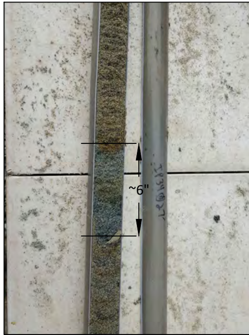
Photograph 13: View of injection point 34 sandy soils at 27 feet bgs (at soil/groundwater interface). Mottled orange and blue-gray contaminated soils (approximately 6-inch horizon) as shown. Photo taken on July 14, 2021. The soil sample collected from the contaminated horizon at 27 feet bgs had a PID reading of 1.5 ppmv.
