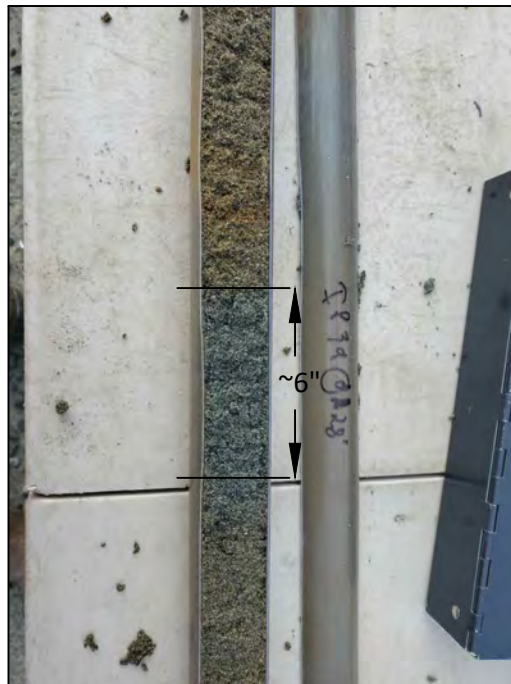
Photograph 12: View of injection point 39 sandy soils at 28 feet bgs (at soil/groundwater interface). Visible blue-gray contaminated soils (approximately 6-inch horizon) as shown. Photo taken on July 14th, 2021. Note: The groundwater grab sample collected from injection point 39, prior to any chemical injections, was non-detect for the contaminants of concern. The soil sample collected from the contaminated soil horizon at 28 feet bgs had a relatively low PID reading of 1.8 ppmv.
