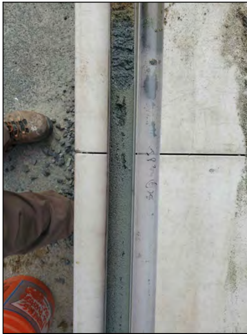
Photograph 15: View of injection point 33 sandy soils at 28 feet bgs (at soil/groundwater interface). Blue-gray contaminated soils had a PID reading of 5,000 ppmv. The contaminated soil horizon was approximately 1 foot in length. Photo taken on July 14th, 2021.
