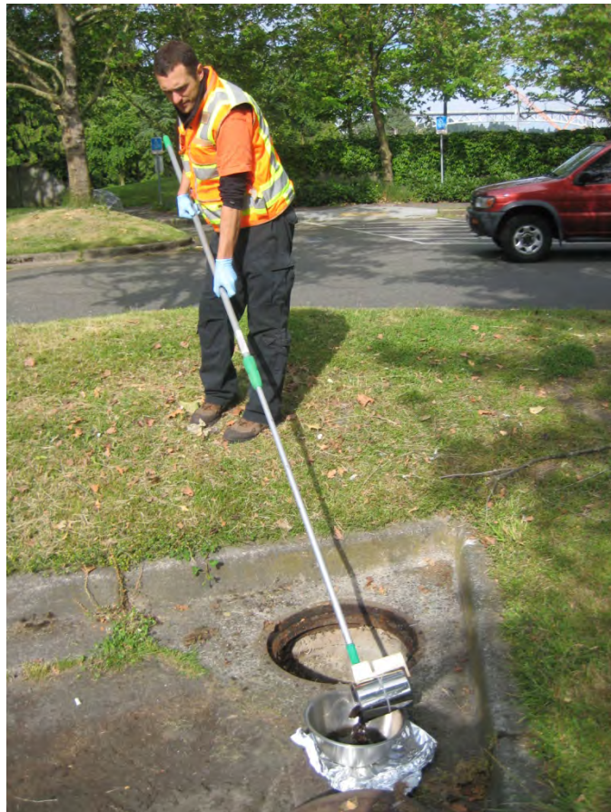
Photo 4. SPU staff sampling Catch Basin PA-CB-02 in Gas Works Park parking area.
