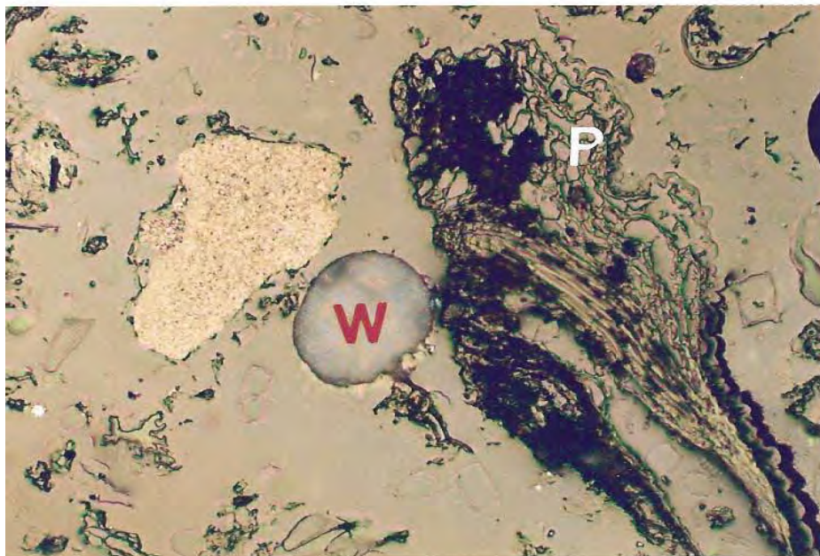
Figure 2: Photomicrographs of Stanford's Sample Labeled NLU-58 Showing; C =Carbon Black Aggregate (dense aggregate), T =Pitch with QI, P =Cellular Plant Material, R =Particulate Plant, M =Metallurgical Coke, W =White Grainy Mineral and E =Epoxy Mounting Media. Reflected Light In Air, X250.
