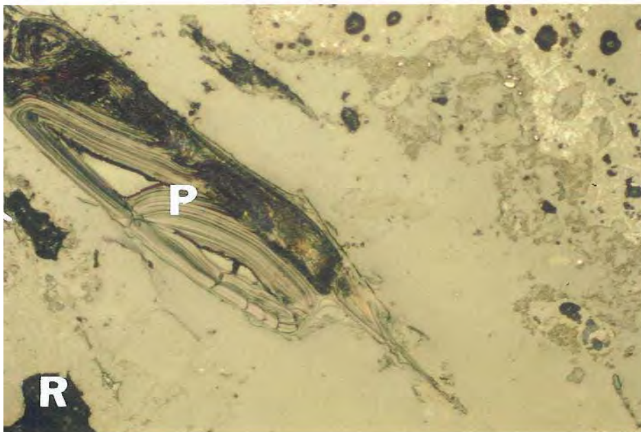
Figure 1: Photomicrographs of Stanford's Sample Labeled NLU-68-52 Showing; C =Carbon Aggregate (loose) P =Cellular Plant Material, R =Particulate Plant, D =Diatomaceous Mass, K =Coal, M =Metallurgical Coke with Pyrolytic Coating, S =Slag, and E =Epoxy Mounting Media. Reflected Light In Air, X250.
