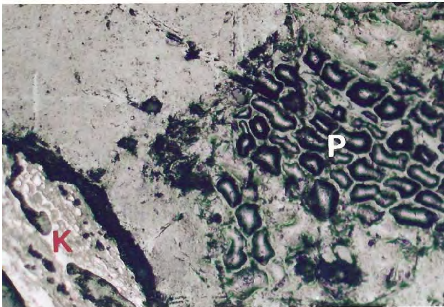
Figure 1: Photomicrographs of Stanford's Sample Labeled NAPL Showing; C=Carbon Black Aggregate in Pitch, T=Pitch (normal), S=Cenosphere, P=Cellular Organic Plant Material, K=Met Coke and L=Slag. Reflected Light In Air, X250.
