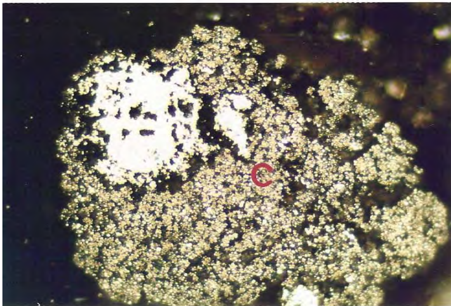
Figure 8: Photomicrographs of Stanford's Sample Labeled NLU-72 Showing; C =Carbon Aggregate (dense and loose), N =Small QI Aggregate, P =Cellular Plant Material, R =Particulate Plant, D =Diatomaceous Mass, A =Diatom and E =Epoxy Mounting Media. Reflected Light In Oil, X600.
