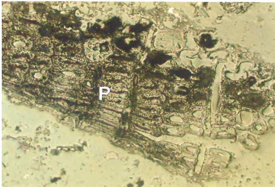
Figure 9: Photomicrographs of Stanford's Sample Labeled NLU-68-51 Showing; P=Cellular Plant Material, R=Particulate Plant, PK=Pitch Coke, K=Coal, S=Slag, Q=Quartz, O=Odd Mineral, U=Rust and E=Epoxy Mounting Media. Reflected Light In Air, X250.
