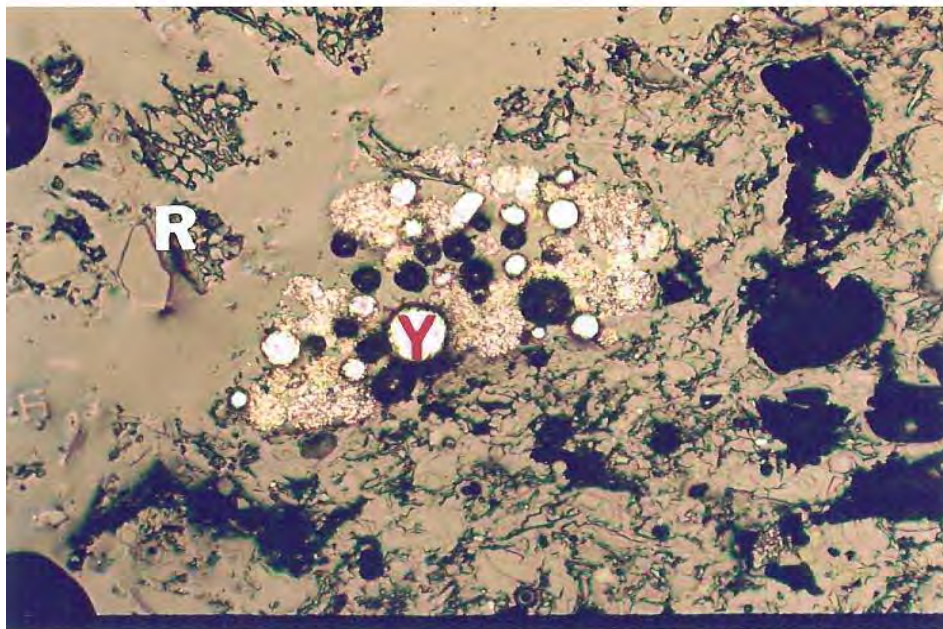
Figure 6: Photomicrographs of Stanford's Sample Labeled NLU-45DC Showing; T=Pitch with QI, P=Cellular Organic Plant Material, R=Particulate Plant, D=Diatomaceous Mass, O=Other Mineral and Y=Pyrite. Reflected Light In Air, X250.
