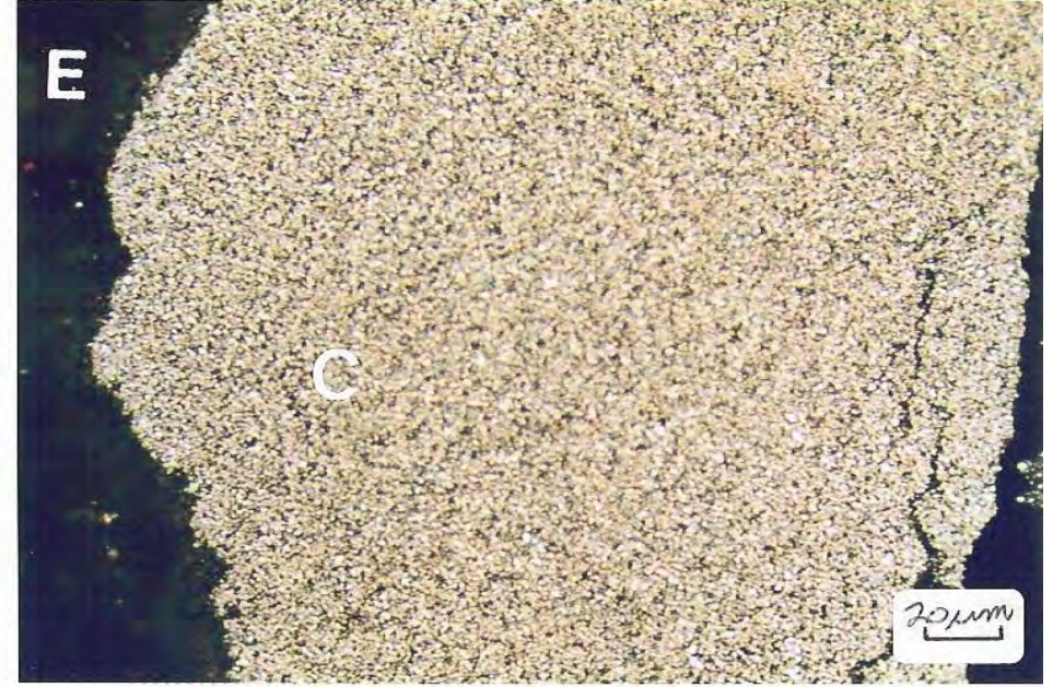
Figure 8: Photomicrographs of Stanford's Sample Labeled NLU-62 Showing; C=Carbon Aggregate (dense), T=Pitch with QI, N=Individual Normal QI, P=Cellular Plant Material, R=Particulate Plant, D=Diatomaceous Mass, A=Diatom and E=Epoxy Mounting Media. Reflected Light In Oil, X600.
