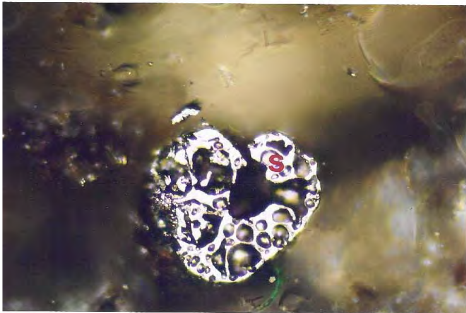
Figure 4: Photomicrographs of Stanford's Sample Labeled NLU-58 Showing; P=Cellular Organic Plant Material, R=Particulate Plant, D=Diatomaceous Mass, A=Diatom, S=Cenosphere and M=Metallurgical Coke with Depositional Carbon (X=Pyrolytic and U=Spherulitic Carbon) Coating. Reflected Light in Oil, 600X.
