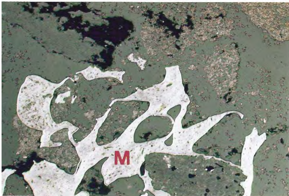
Figure 5: Photomicrographs of Stanford's Sample Labeled NLU-65 Showing; C=Carbon Black Aggregate (loose), N=Individual QI, U=Spherulitic Carbon, P=Cellular Organic Plant Material, R=Particulate Plant, K=Coal and M=Metallurgical Coke. Reflected Light In Air, X250.
