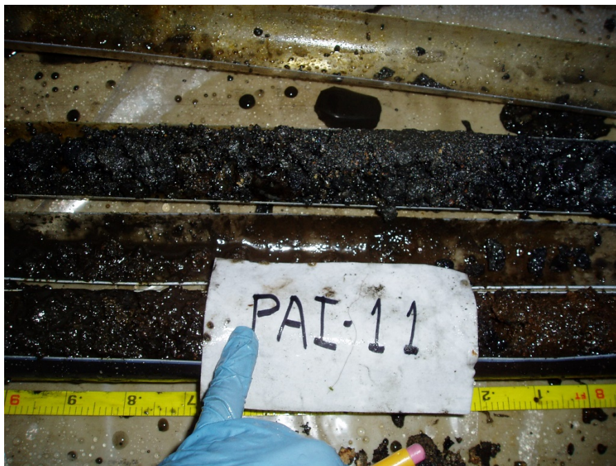
PAI-11 11 to 14 feet top (back) liner
