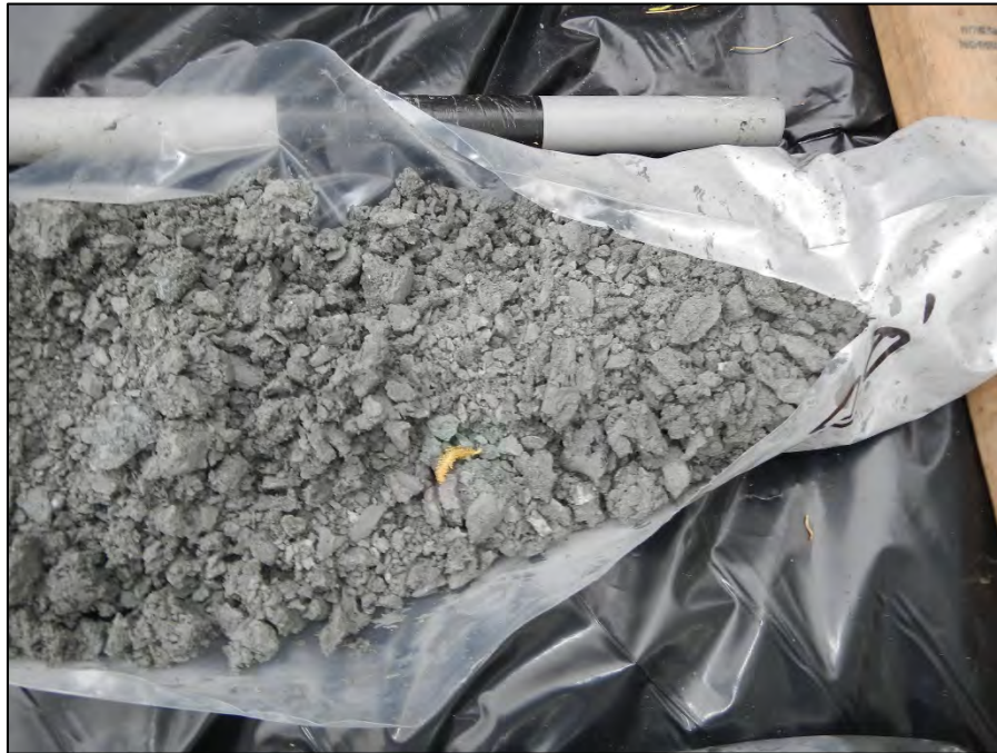
MW-40S 15 to 20 feet
