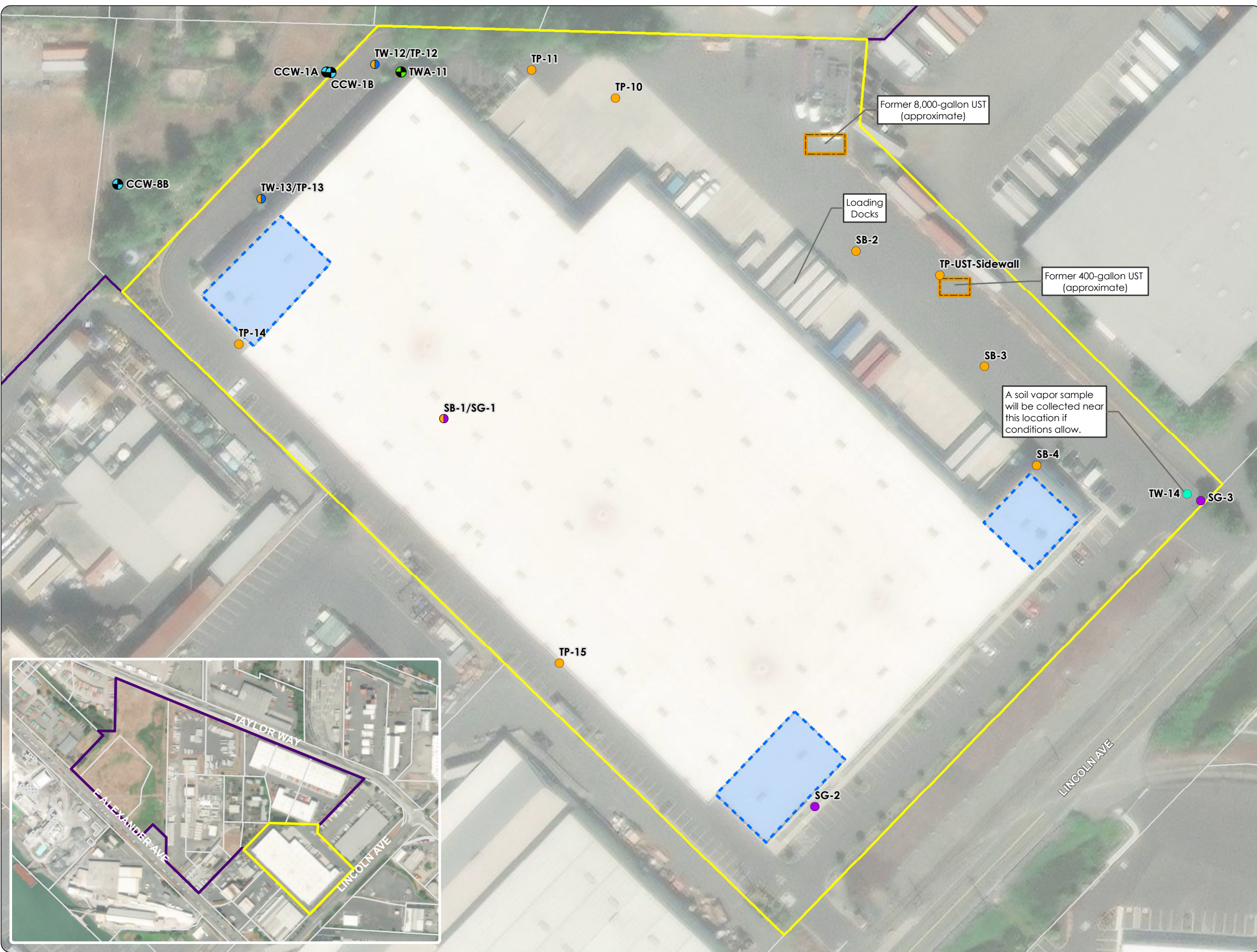
Figure 1 Parcel 110 Property Features and Proposed Sample Locations Port of Tacoma TWAFA Site Tacoma, Washington
