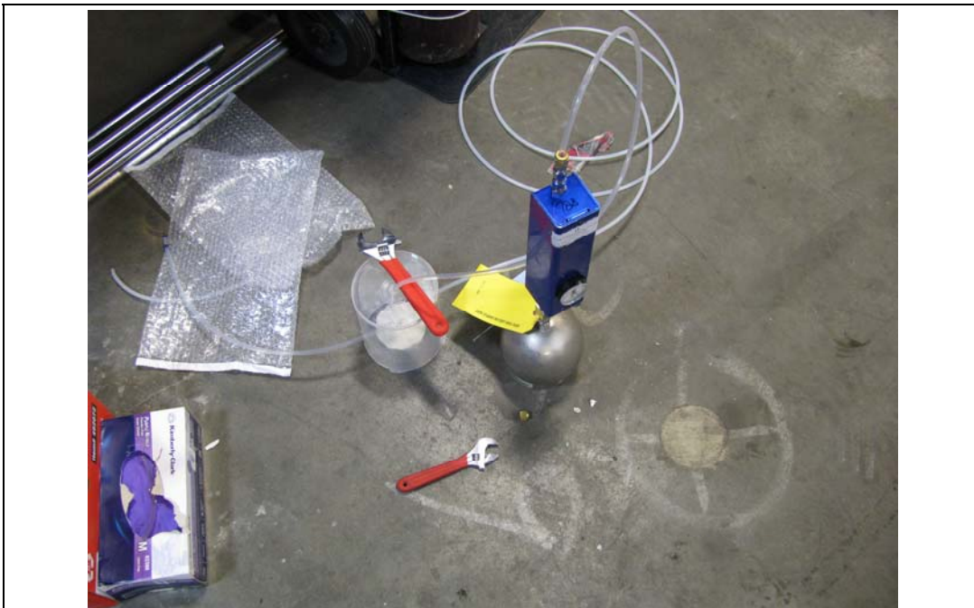
Photograph No: 2 Sub-slab soil vapor sampling train set up at SSV-B
