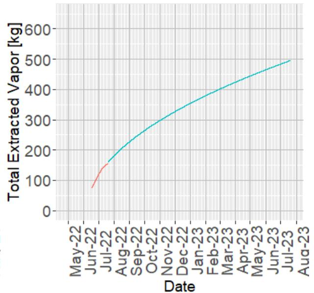
Note: The air sparging mass forecasts shown here start with the total extracted VOC mass in vapor prior to start of sparging (about 100 kg).
