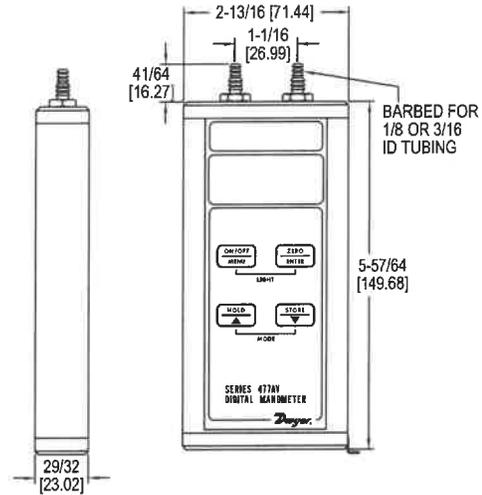
The Series 477AV Handheld Digital Manometer is now available with pressure, flow, and velocity measurements along with a number of other convenient features. The built-in air velocity and flow calculations provide accuracy and conserve time and error associated with manual calculations. Also featured on this unit are adjustable zero and span values for calibrating in the field, as well as a damping feature to compensate for the fluctuating of readings.
