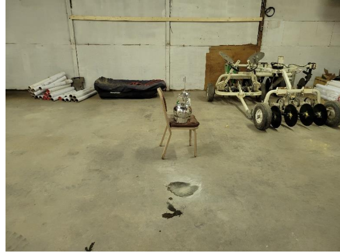
Photo 6. View of indoor air sample collected in 6-liter summa cannister inside warehouse. Photo taken on 5/11/2022.
