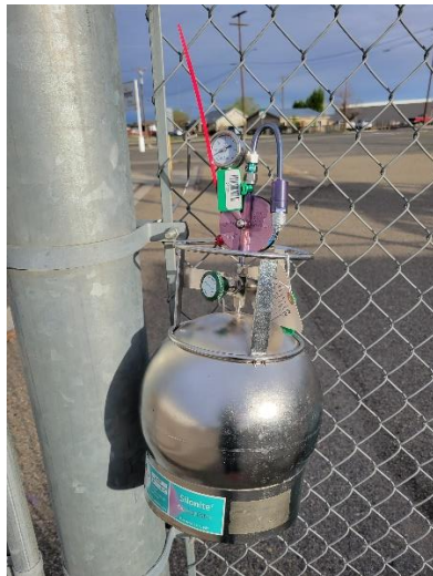
Photo 11. View of ambient air sample collected outside on fence between warehouse and modular office building. Photo taken on 5/11/2022.
