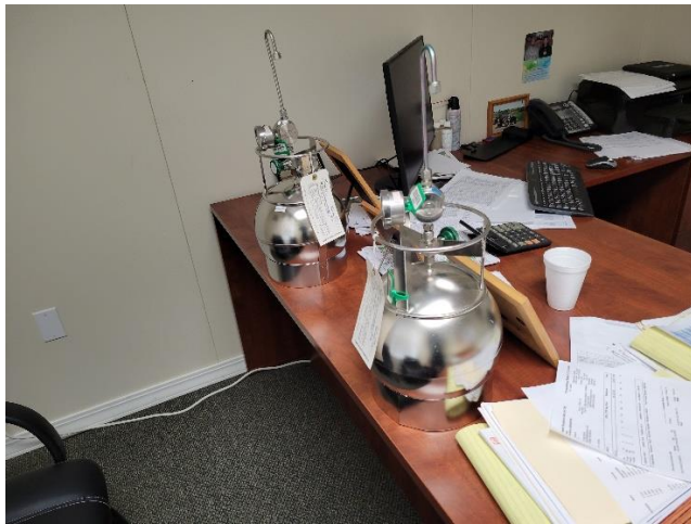
Photo 9. View of indoor air sample and duplicate sample collected from modular office building interior. Photo taken on 5/11/2022.
