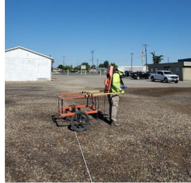
Figure 2. Geonics EM61 Time Domain Metal Electromagnetic Induction Metal Detector (TDEMI)
