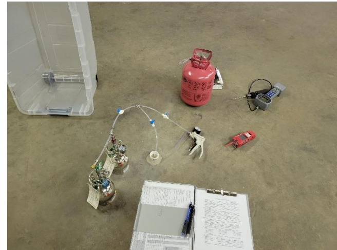
Photo 4. View of subslab vapor sample collection in warehouse. Photo taken on 5/11/2022.
