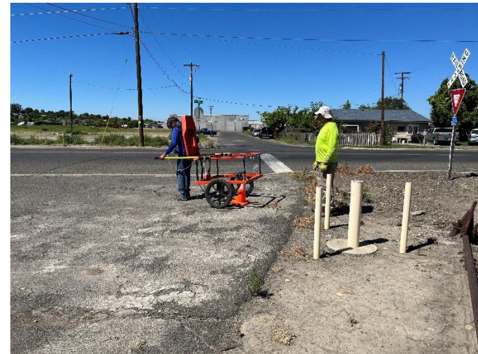
Photo 12. View of ground penetrating radar equipment used during geophysical survey. Photo taken on 8/16/2022.
