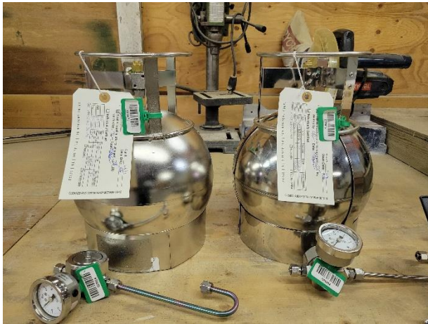
Photo 7. View of indoor air samples collected from warehouse in 6-liter summa cannisters. Photo taken on 5/11/2022.
