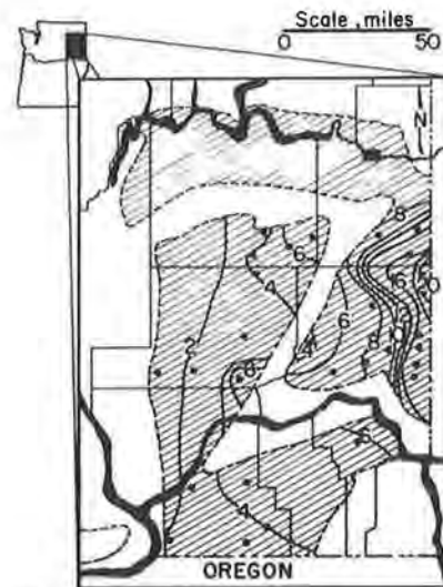
FIGURE 10 Generalized contour map of percentage content of clay-size particles for southeastern Washington loess.
