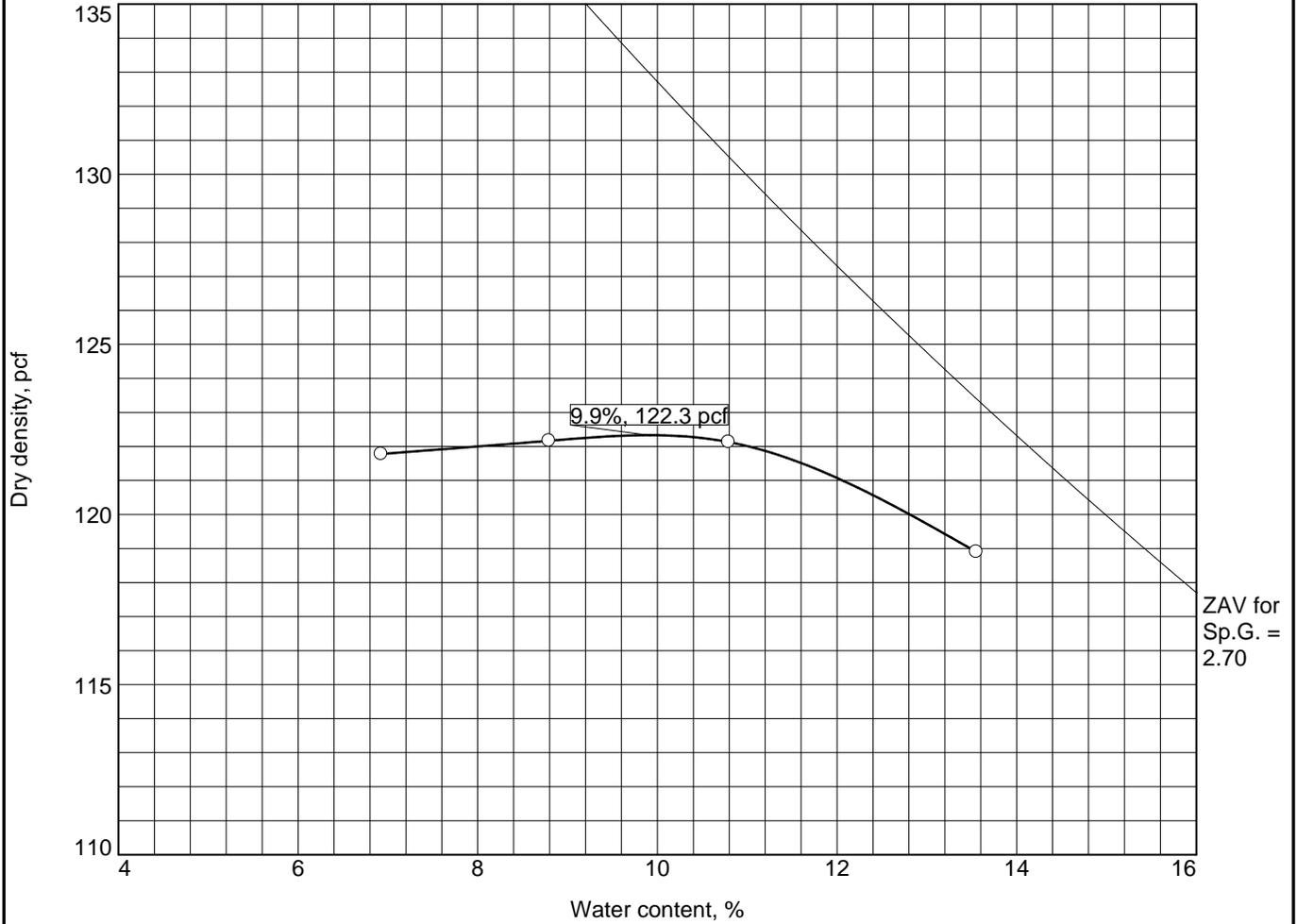
Test specification: ASTM D 1557-02 Method A Modified
