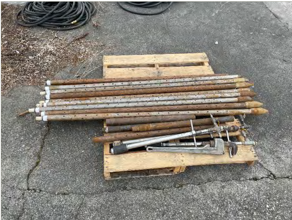
Exhibit 6-3: Photo of Several 5-Foot Injection Tools
