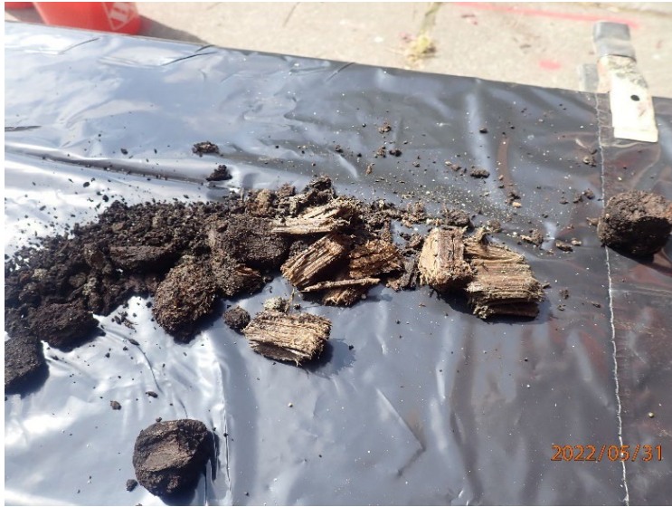
Close-up view of organics (wood fragments and peat) encountered below a depth of 4 feet at EMW01.
