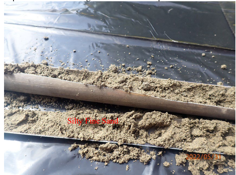
Close-up view of poorly-graded sand with gravel encountered in upper 4 feet at EMW01.
