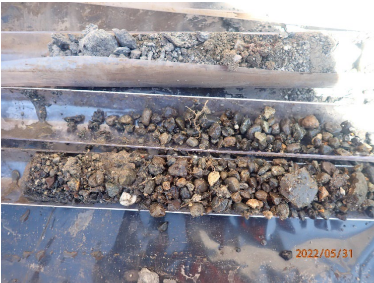
Pea gravel encountered in EB05 is likely backfill from previous remedial excavations. Fill and underlying native soils were sampled.
