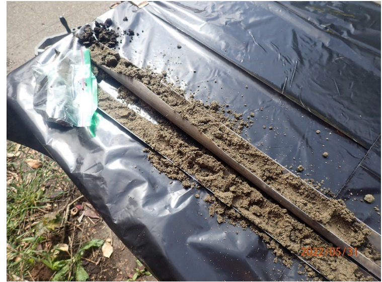
Soil cores retrieved inside 4-foot-long plastic sleeves were accessed to perform field screening and collect soil samples.
