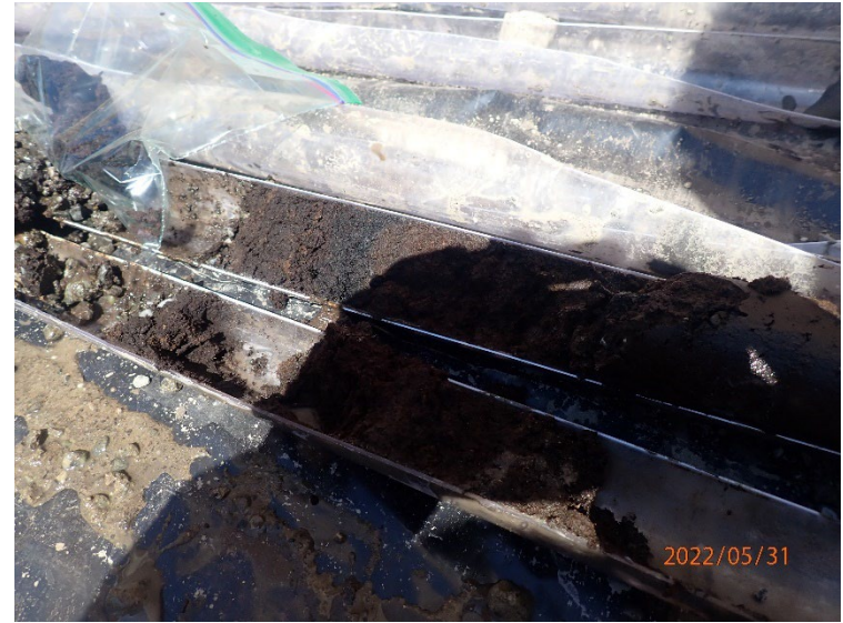
About 15 inches of peat was encountered beneath the pea gravel fill.
