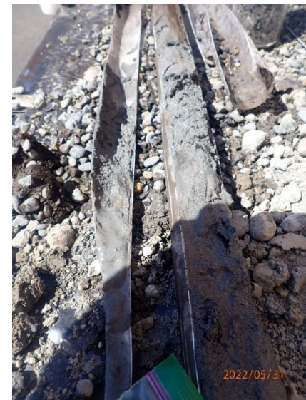
The peat layer was underlain by about 2.5 feet of saturated sandy silt extending to the termination depth of 16'.
