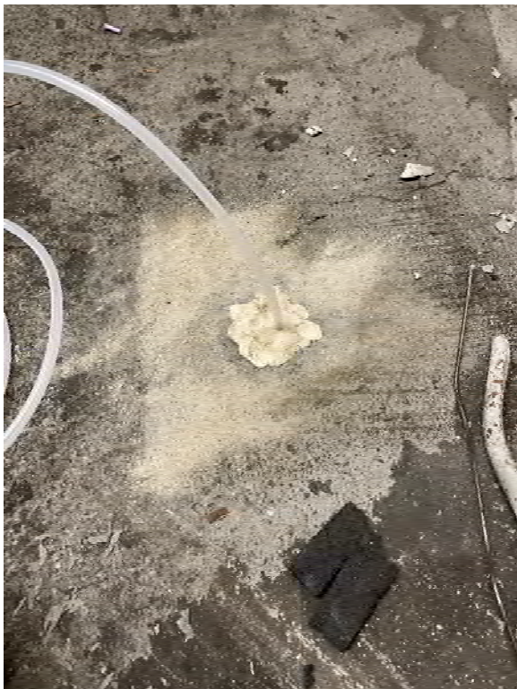
SV-3 Sub-Slab Sample Location – Tube in place with modeling clay
