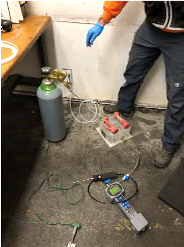
SV-3 Sub-Slab Sample Location – Sealed with Cement Post Sampling
