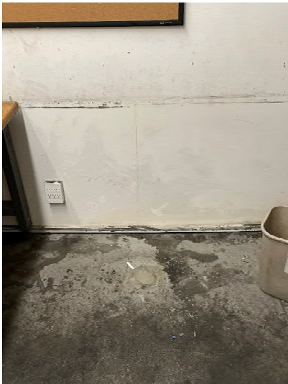
SV-3 Sub-Slab Sample Location – Sealed with Cement Post Sampling
