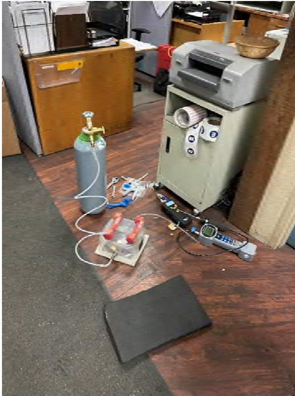
SV-2 Sub-Slab Sample Location – Summa Canisters with Duplicate “T”
