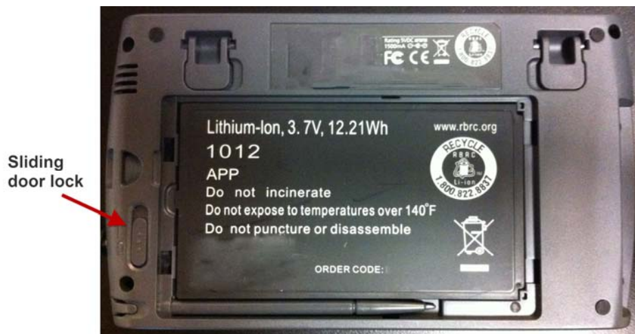
LabNavigator with battery door removed
