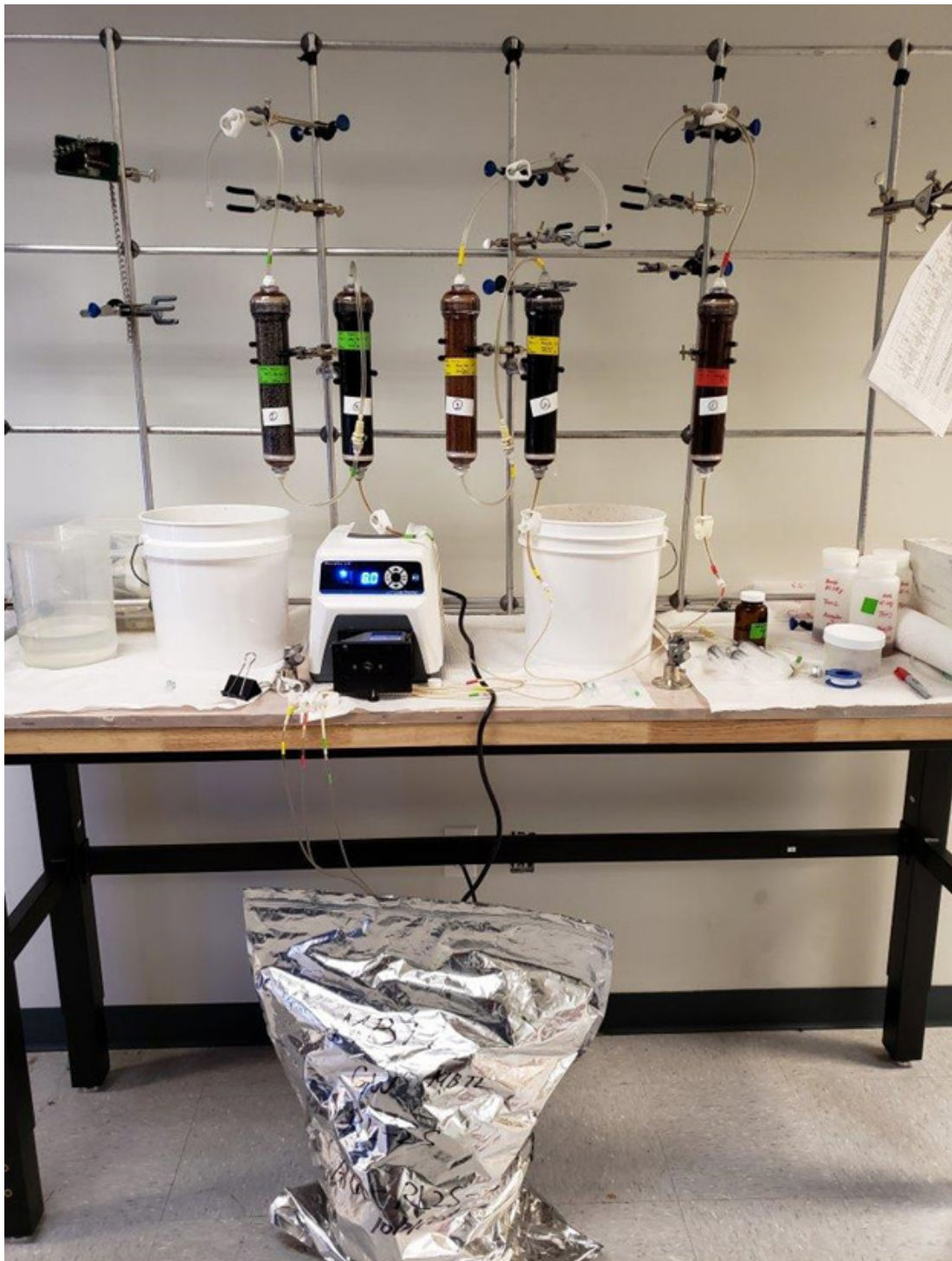
Figure 16 Column Test Equipment Setup
