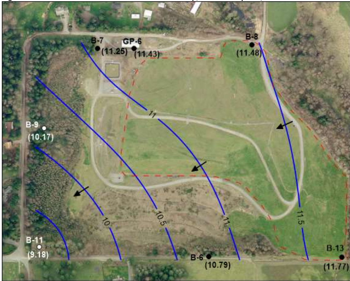
Figure 3d. Potentiometric Surface Contour Map, Perched Aquifer, December 2021.
