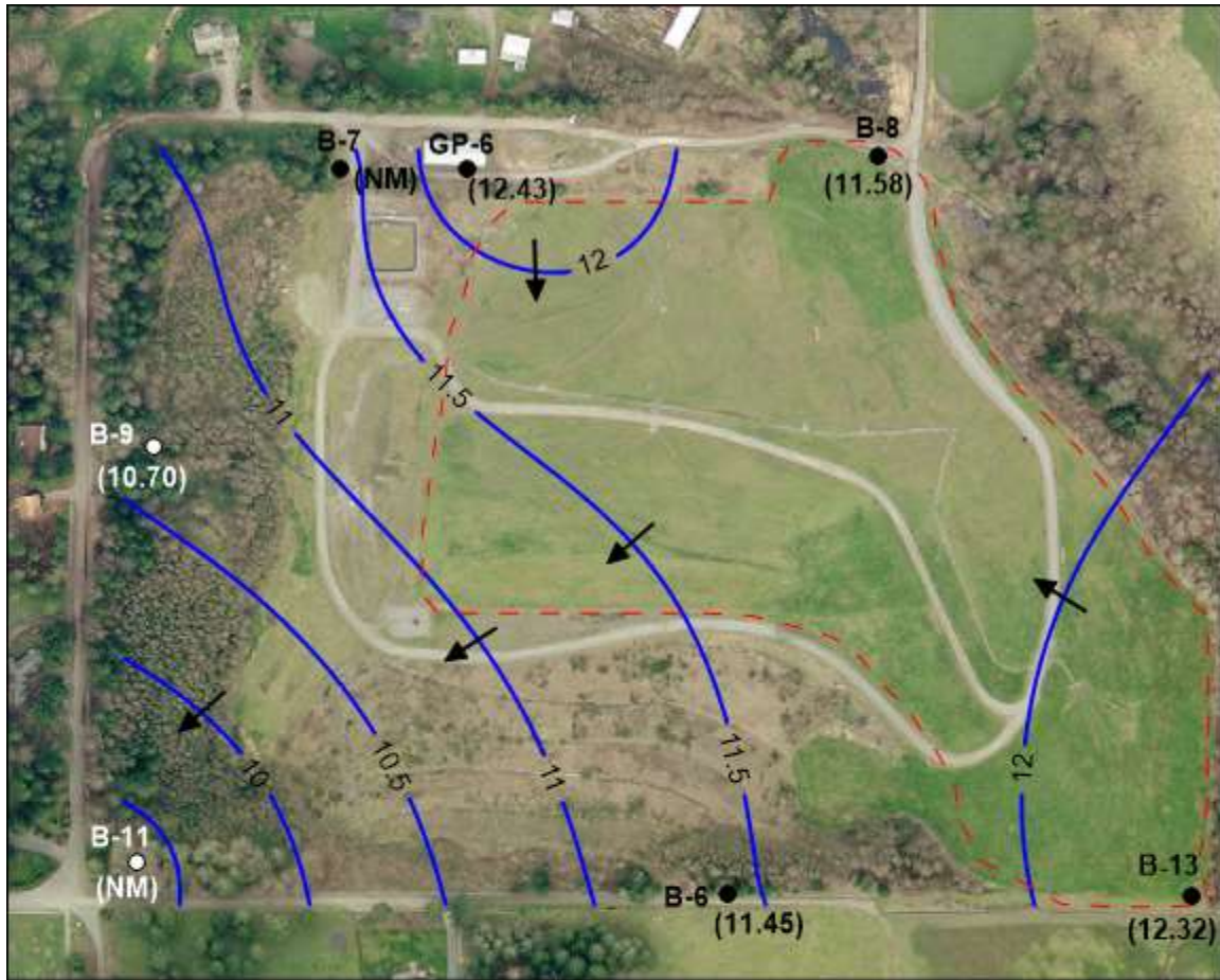
Figure 3b. Potentiometric Surface Contour Map Perched Aquifer, June 2021.
