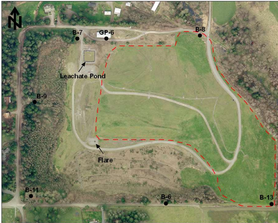
Figure 3. Perched Aquifer Monitoring Well Locations.
