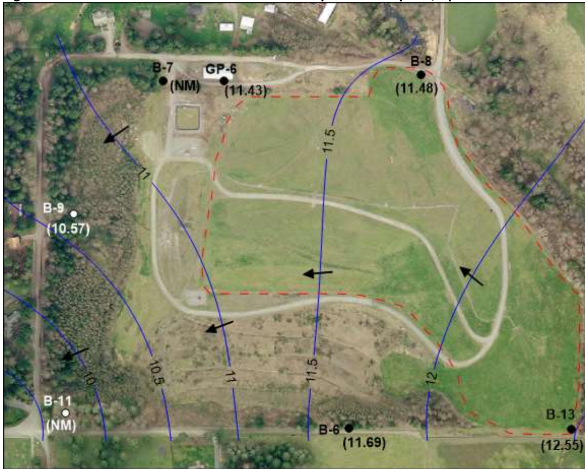
Figure 3a. Potentiometric Surface Contour Map Perched Aquifer, April 2021.
