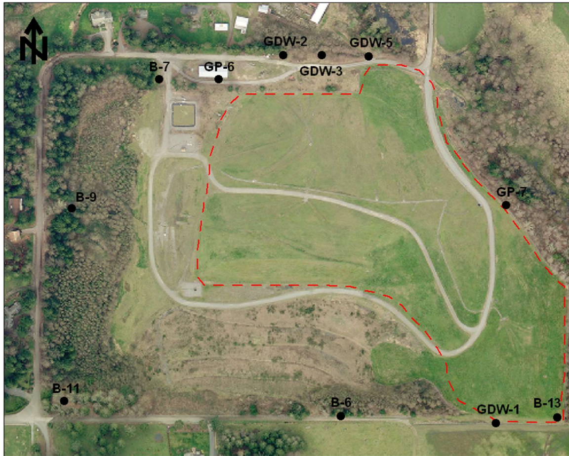
Figure 9. Landfill Gas Perimeter Monitoring Probe Locations.
