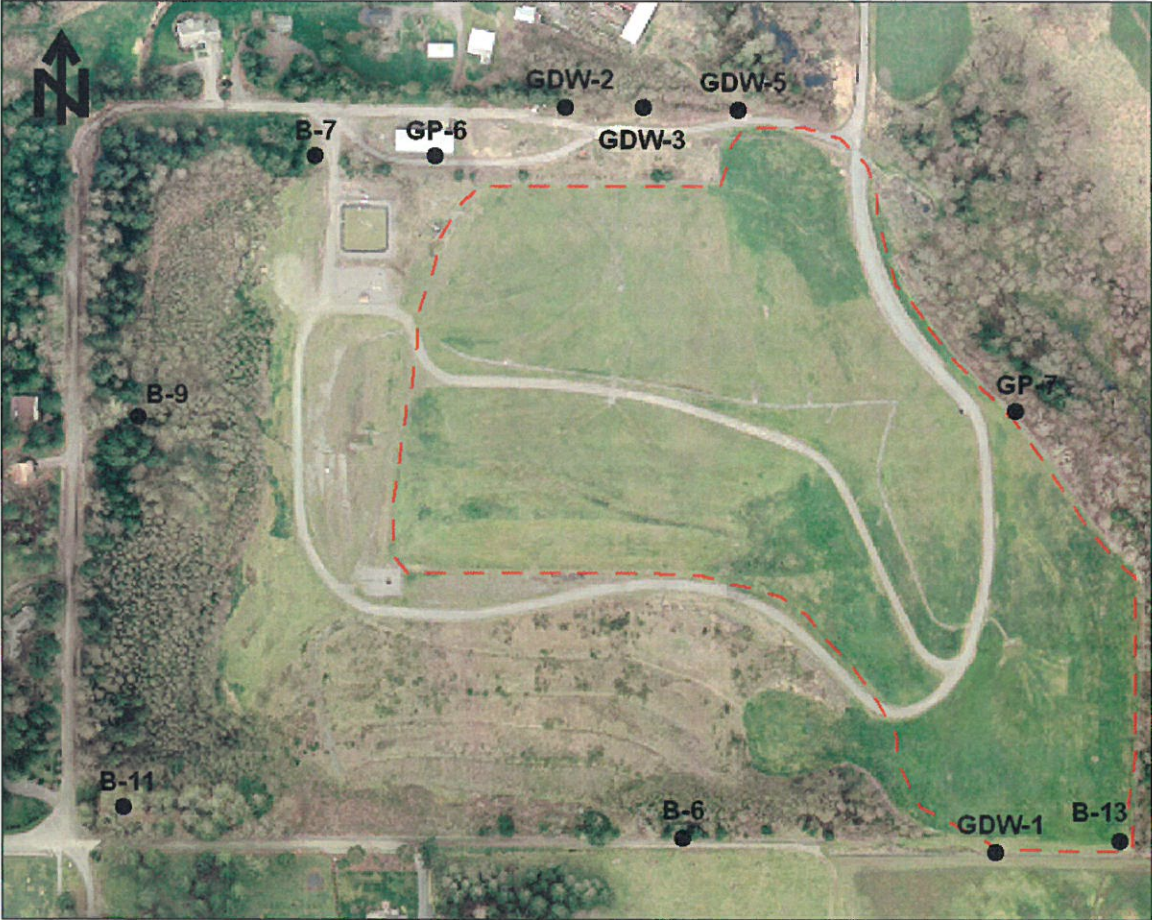
Figure 9. Landfill Gas Perimeter Monitoring Probe Locations.
