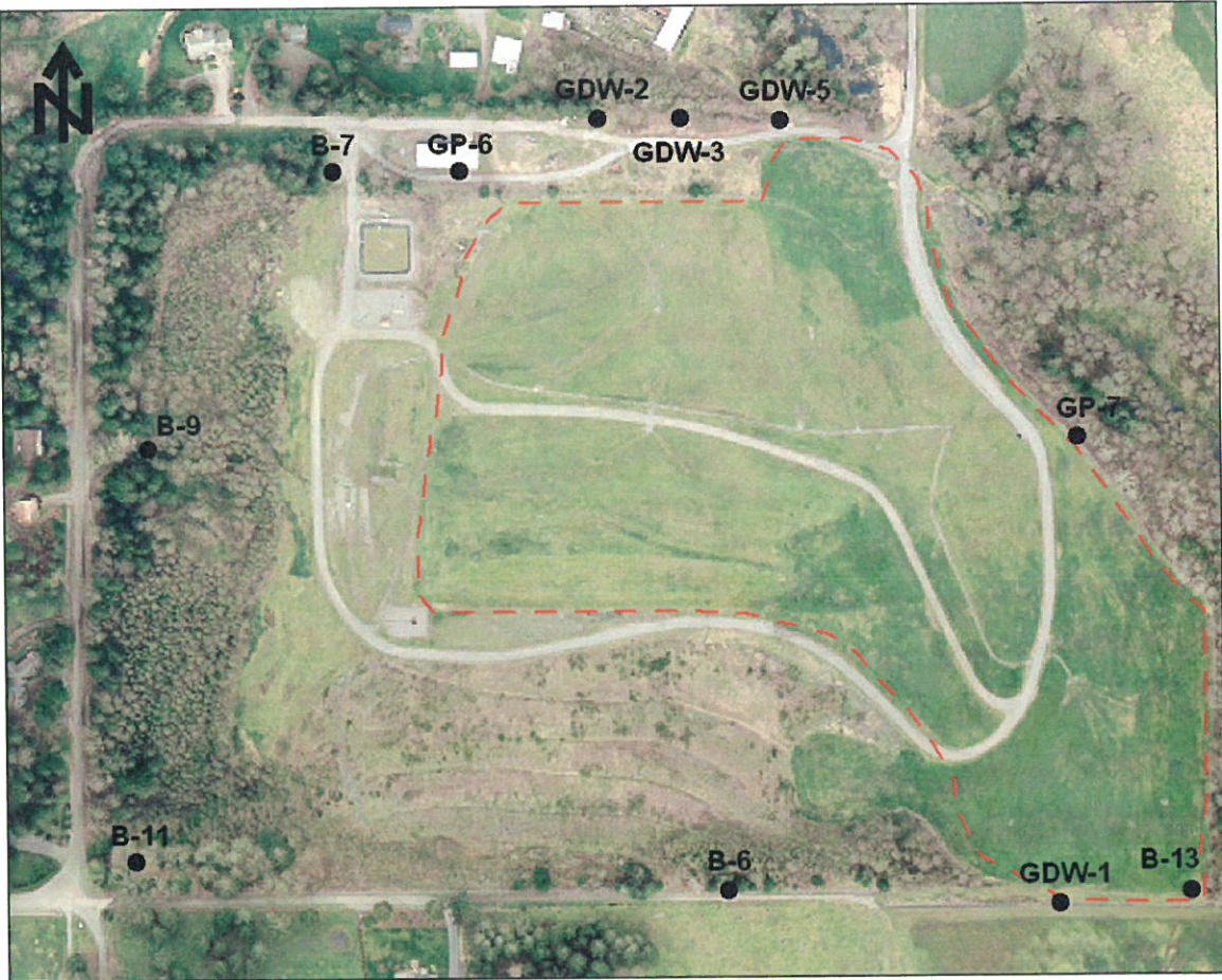
Figure 9. Landfill Gas Perimeter Monitoring Probe Locations.
