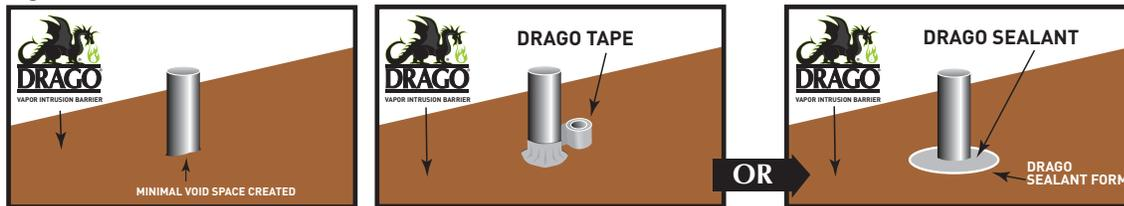
Fig. 4b: DETAIL PATCH FOR PIPE PENETRATION SEALING
