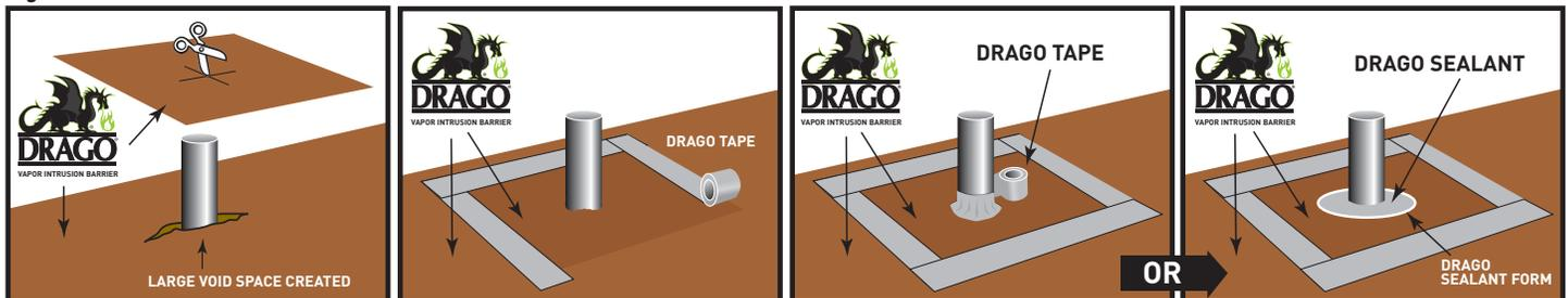
**DETAIL PATCH FOR PIPE PENETRATION SEALING: (Fig. 4b)**
