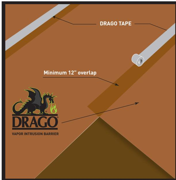
2. Unroll Drago Wrap over the area where the slab is to be placed. Drago Wrap should completely cover the concrete placement area. All joints/seams should be overlapped a minimum of 12 inches and taped using Drago® Tape. (Fig. 1). If additional protection is needed, install DragoTack™ Tape in between the overlapped seam in combination with Drago Tape on top of the seam.
