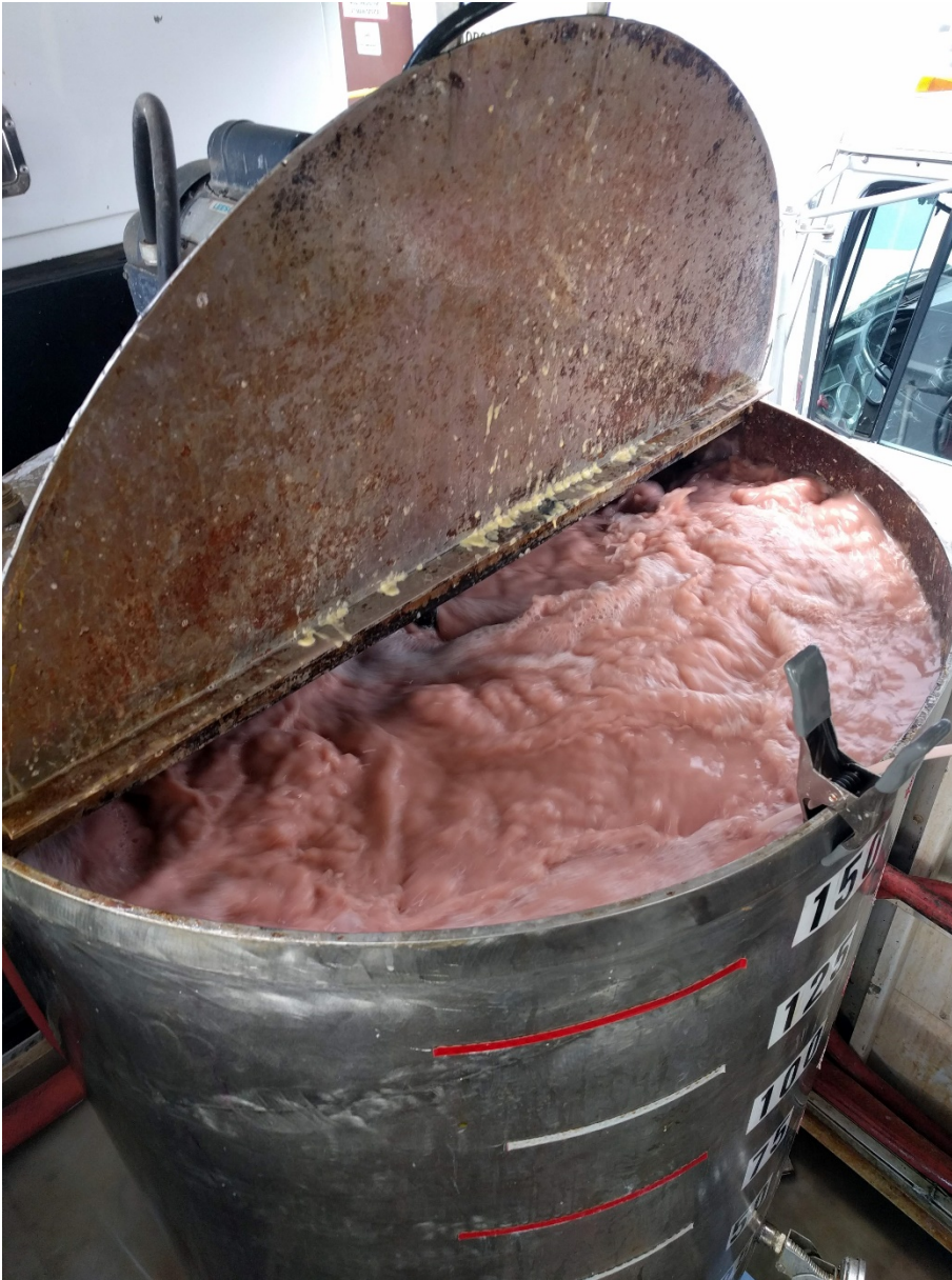
Photograph 3. Injection reagent during mixing.
