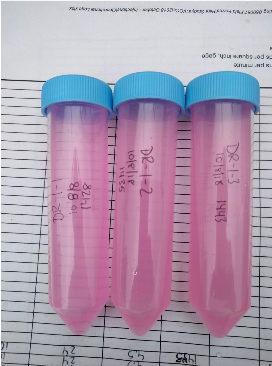
Photograph 4. Grab samples from dose-response wells during injections, showing visual identification of fluorescent tracer.
