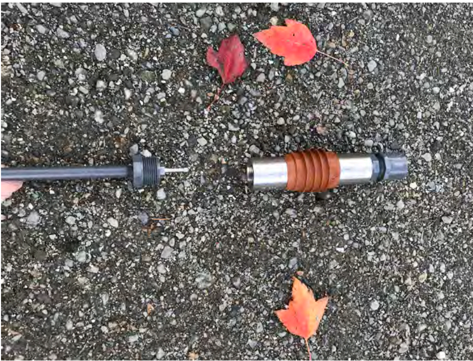
Photograph 12 Date: 11/05/22 Closer view of the Viton K-packer assembly
