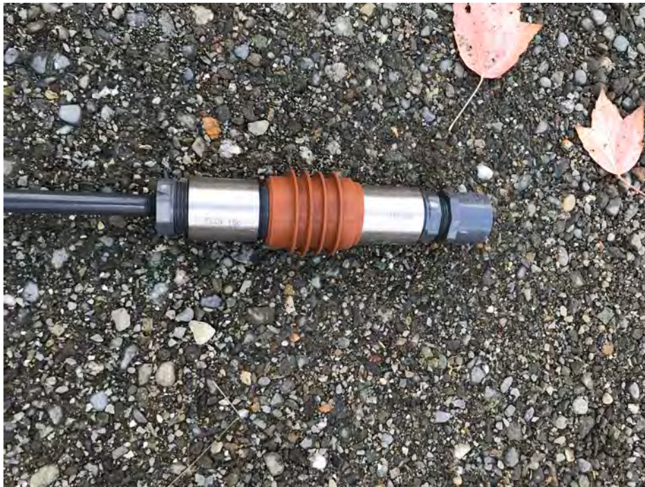
Photograph 11 Date: 11/05/22 Closer view of the Viton K-packer assembly
