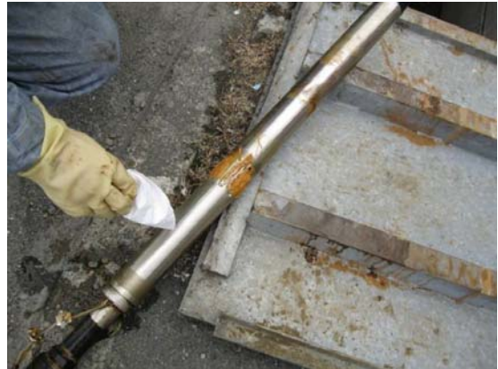
Figure 10. EW-3 pump showing iron precipitate that accumulated on pump intake.
