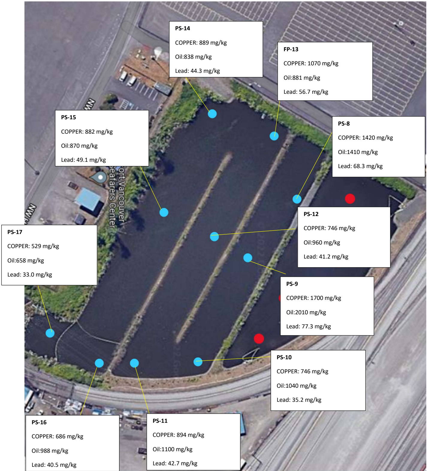
Figure 4 Terminal 4 Stormwater Treatment Facility Additional Forebay Sediment Investigation
