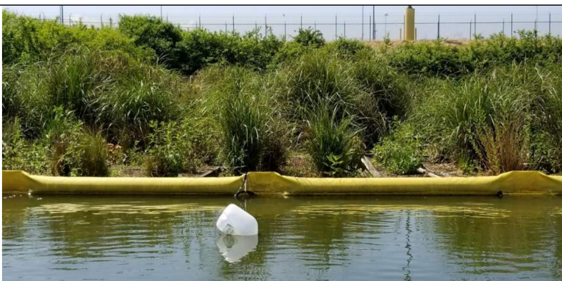
Photo #20: Initial probe deployment from 21 May 2019, the probe floats below the white jug to the right of the FTWs
