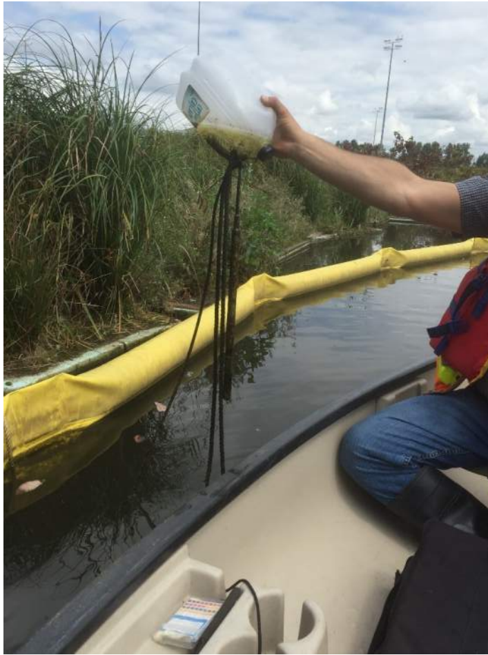
Photo #22: Probe recovery on 16 July 2019; note the layer of green biological growth on the black probe
