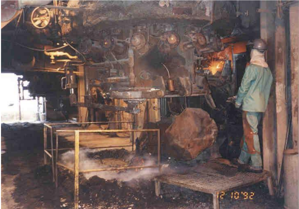
Image Description: Rockwool production at U.S. Gypsum in Tacoma
