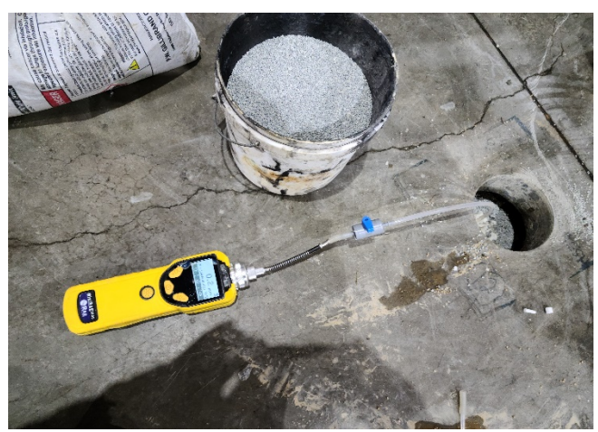
18. Screening soil gas with PID.
