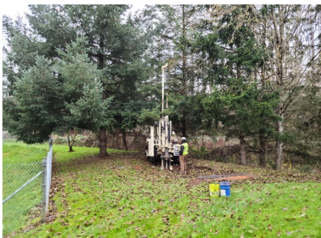
11. Collecting soil samples along the northeast side of the building.
