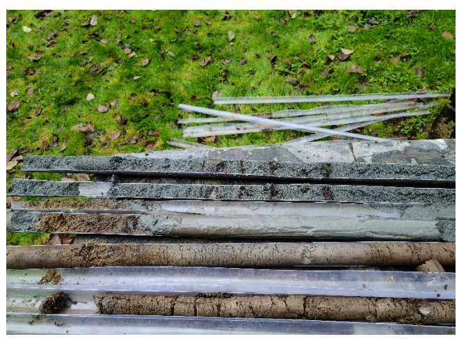
12. Typical soil lithology collected from soil borings.
