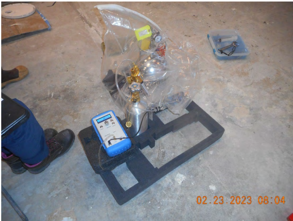
Photograph 4. Sub-slab Sample SV-04 Collection (February 23, 2023)
