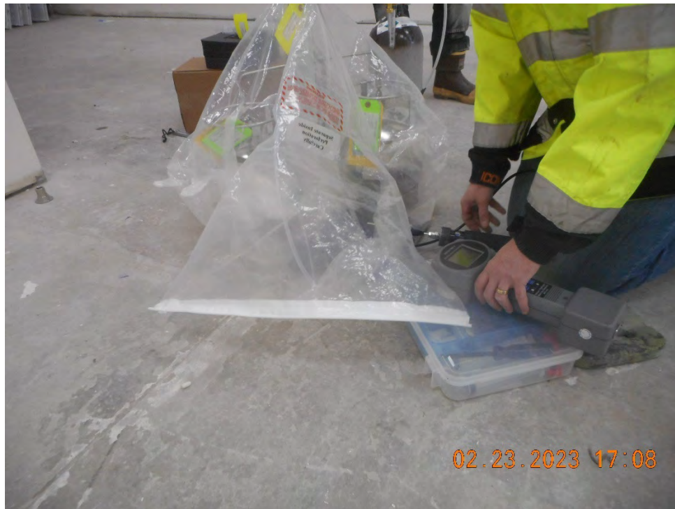
Photograph 5. Sub-slab Sample SV-01 and DUP-01 Set-Up (February 23, 2023)
