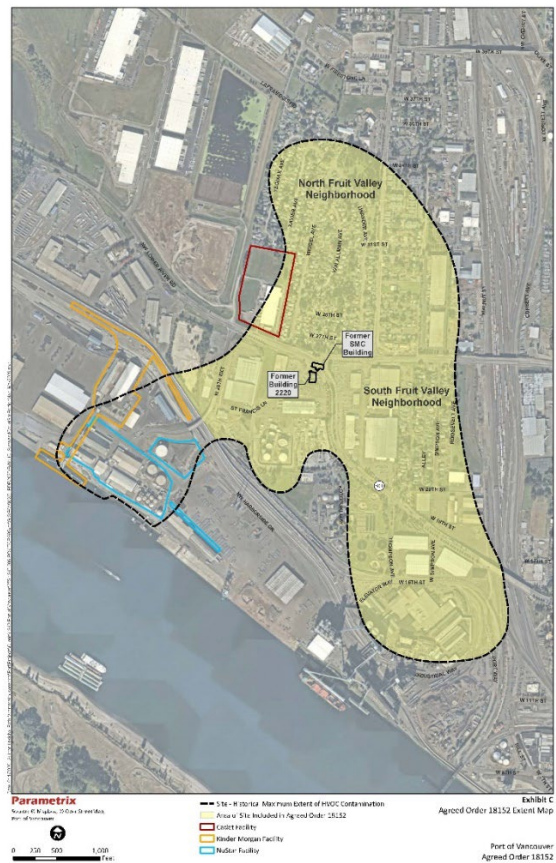
Figure 2. The site is divided into two portions; non-shaded and yellow-shaded. The black line shows the historical maximum extent of solvent contamination prior to interim cleanup actions. The yellow shaded area within the Site outline is the area considered in the AO for partial cleanup by the Port.
