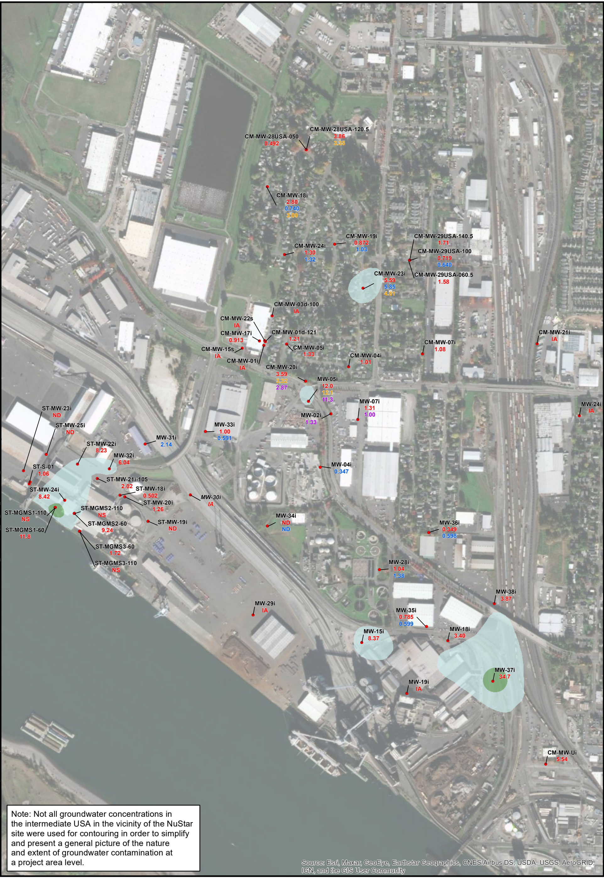
Figure 2-4 2020 TCE Isoconcentrations in Intermediate USA Zone Groundwater
