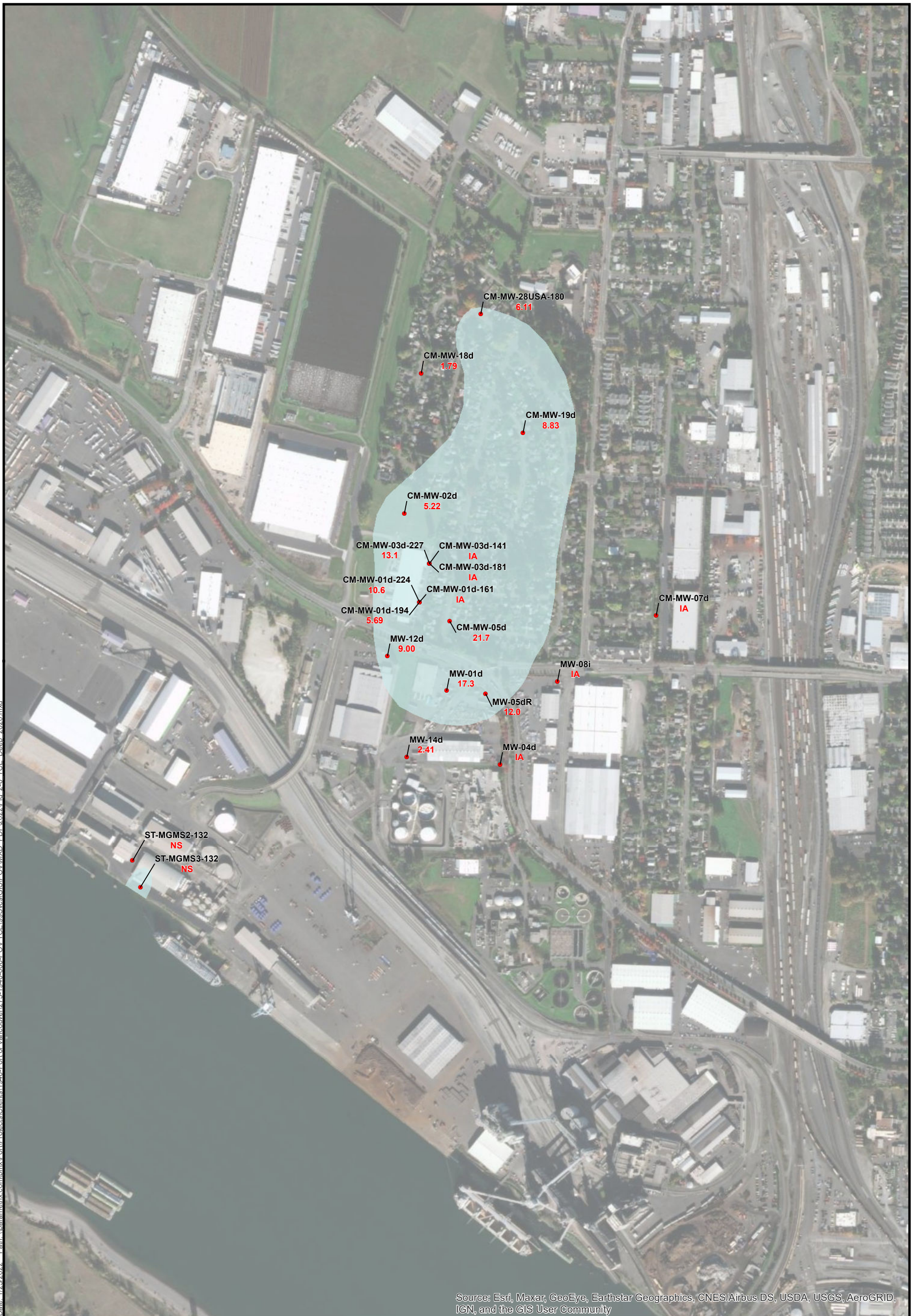
Figure 2-6 2020 TCE Isoconcentrations in Deep USA Zone Groundwater
