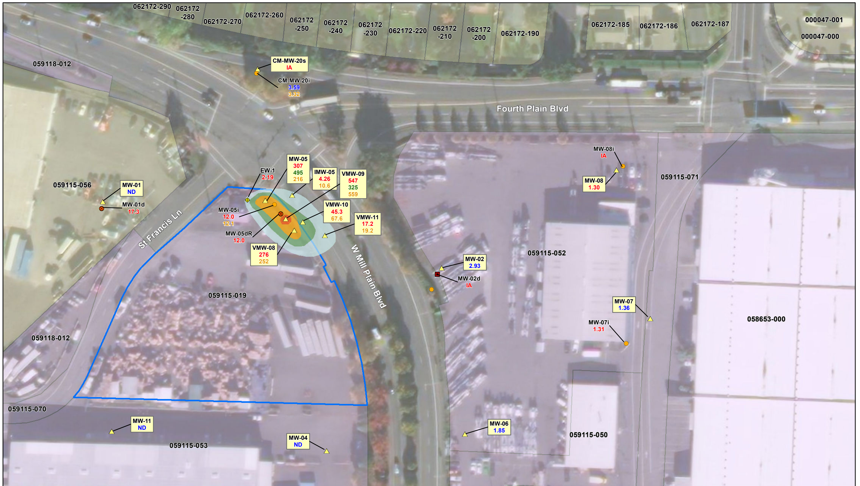
Figure 2-2 Former SMC Site Area TCE Concentrations in Groundwater 1st Quarter 2020
