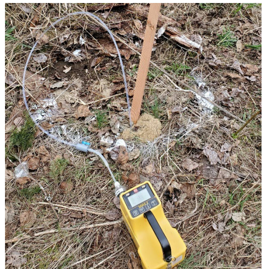
Photo number 4: soil vapor probe monitoring with meter.
