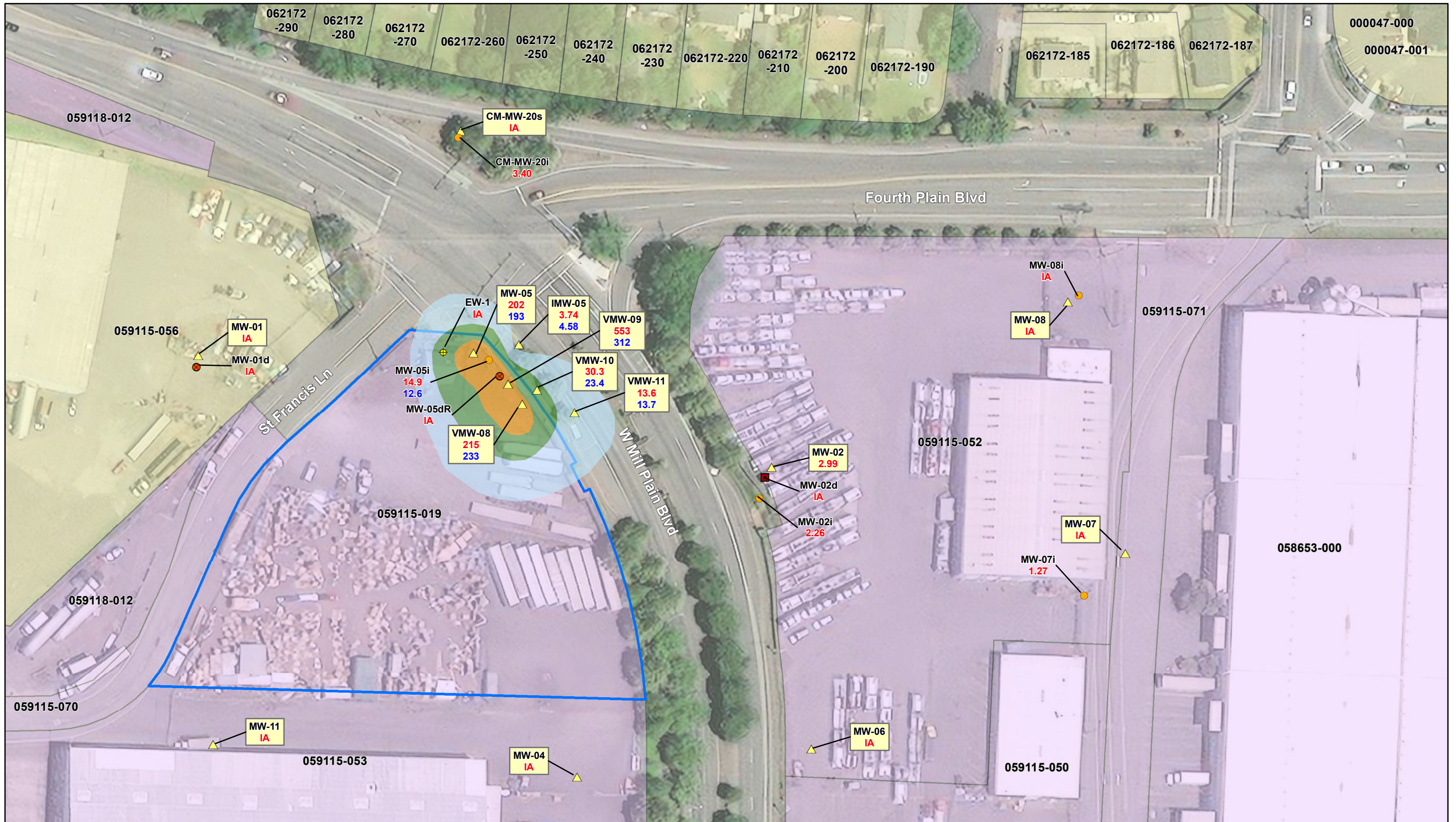
Figure 4-7 Former SMC Site Area TCE Concentrations in Groundwater
