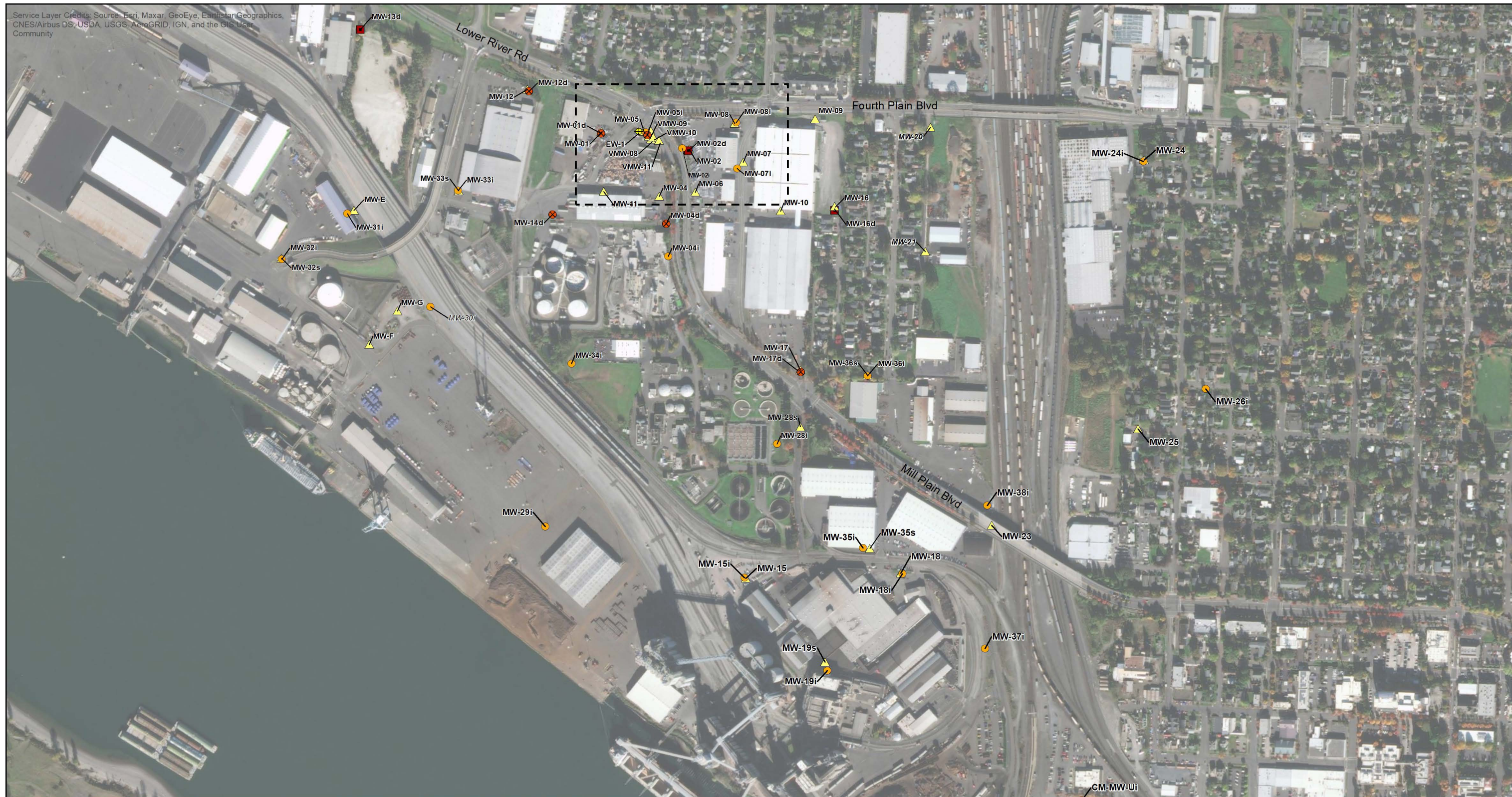
Figure 2-1 SMC Site Groundwater Monitoring Well Locations
