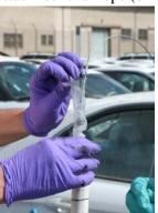
6) Install PFMs by setting transport tube over monitoring well and using Geoprobe rods to push
