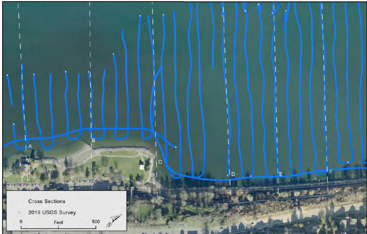
Figure 23. USGS 2019 bathymetry survey track lines.
