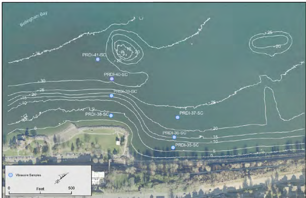
Figure 29. Vibracore sample locations. Imagery Whatcom County 2019. Elevation source DEA 2021 in FT NAVD88.
