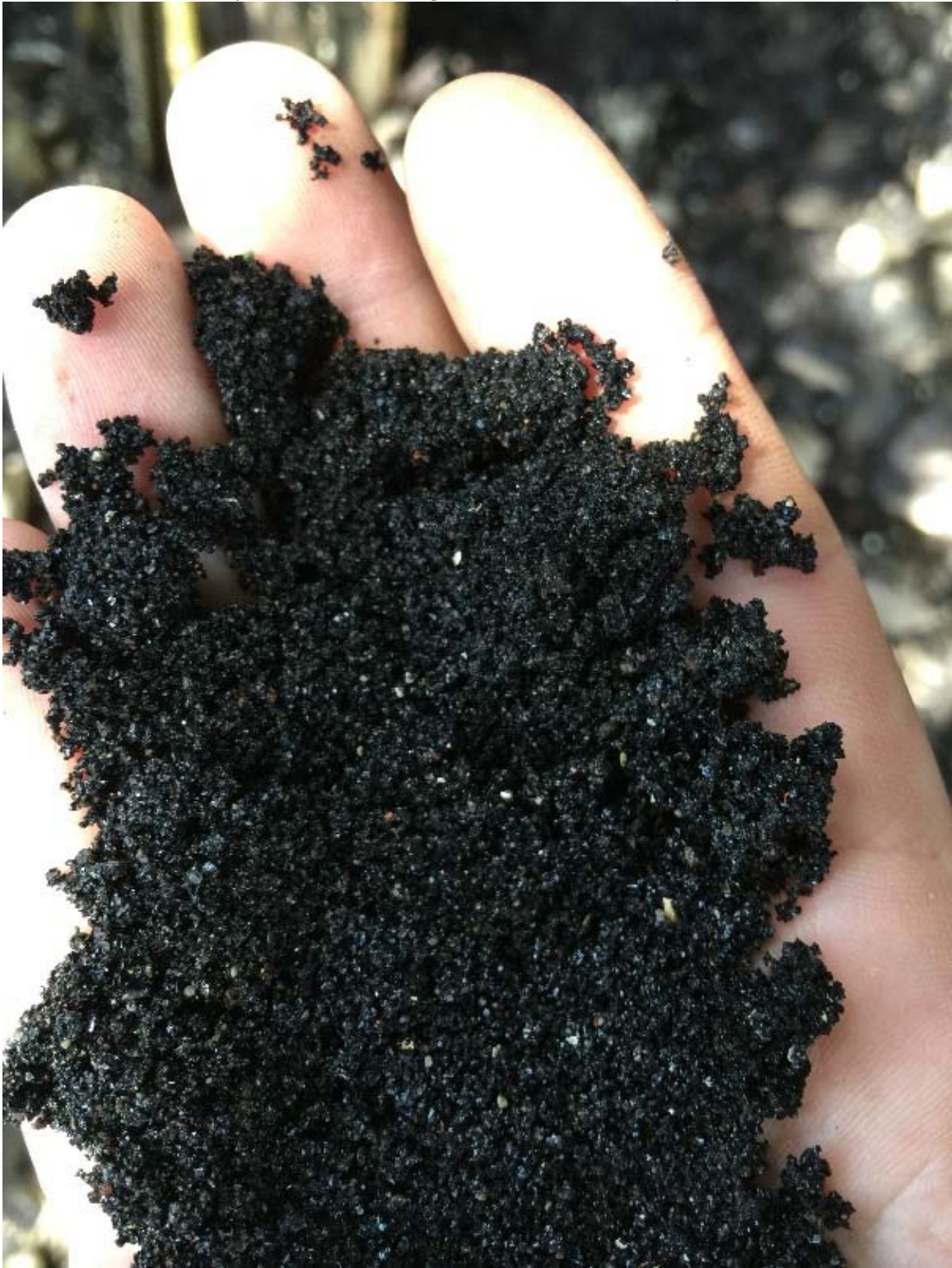
Spent SBG, containing flecks of red and white paint.
