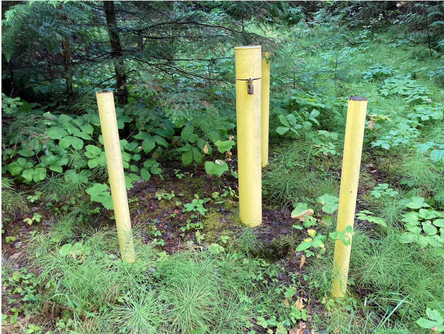
Photo 9: MW-301 as a representative Site monitoring well
