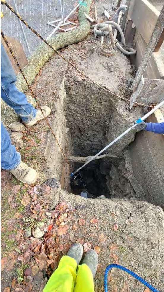
Figure 2. Sampling method, a garden trowel attached to an extendable pole to break up the soil with a lined bucket under it to catch the soil for sampling.
