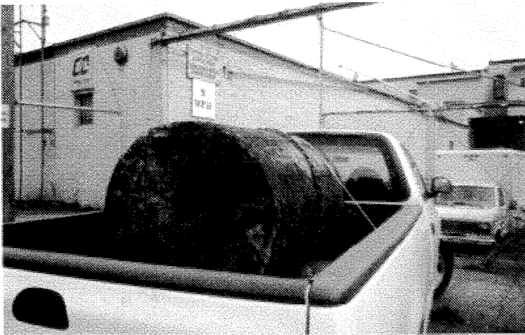
Removed diesel UST with heavy corrosion and several holes.
