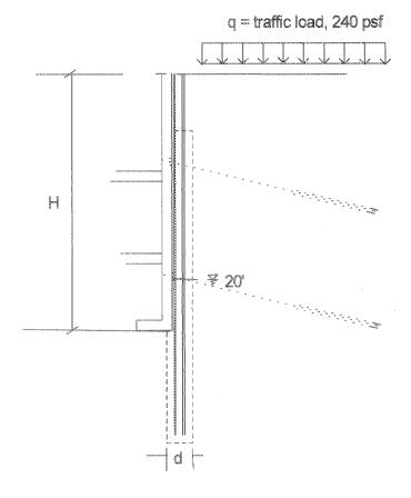
Noe: Assumes permanent dewatering Soil Parameters are design values. Apply Factor of Safety of 1.5 for overturning and kick out.
