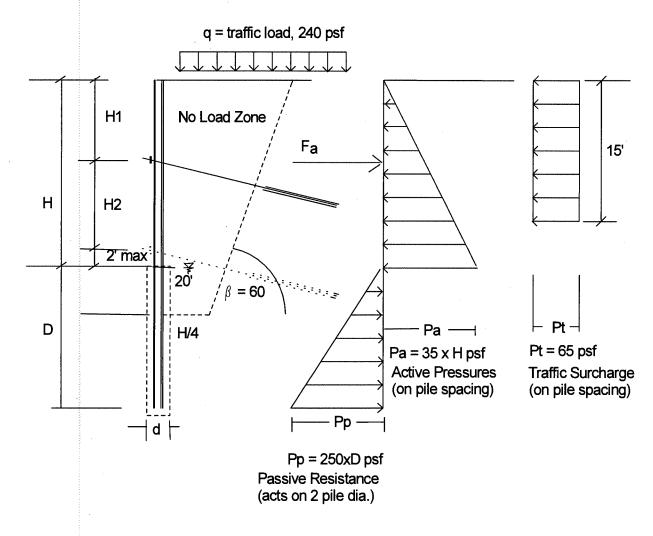
Pressure Grouted Tieback Design Parameters
