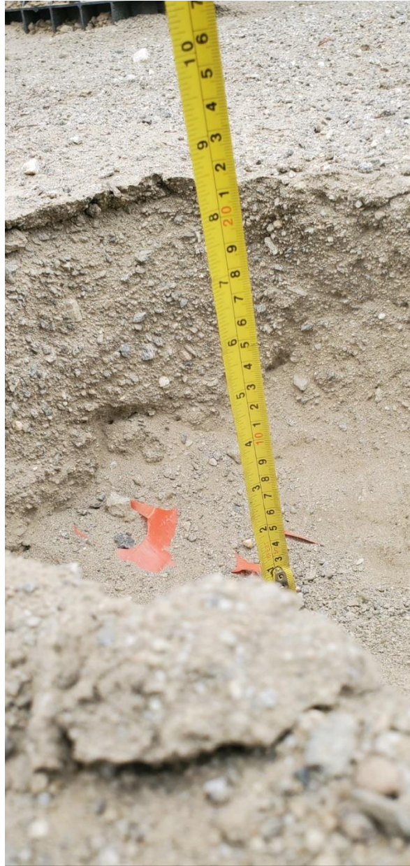
Photograph 7. Depth of clean soils over the marker barrier exceeds 6 inches of depth.
