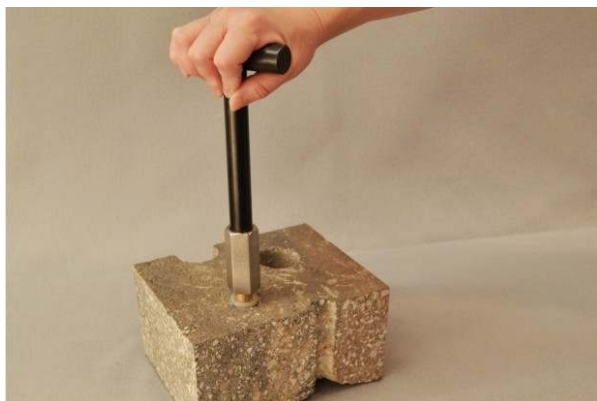
Figure 7. Removing the Vapor Pin™.
