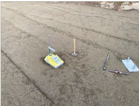
Exhibit E-9: Photos of Compaction Activities. Clockwise From Top-Left: Photo of Excavator Compacting Quarry Spalls in Area 5. View Direction is Southeast. Top-Right: Photo of Smooth-Drum Vibratory Roller in Area 1. View Direction is North. Bottom-Right: Photo of Walk-Behind Vibratory-Plate Compactor in Area 6. View Direction is Southwest. Bottom-Left: Photo of Nuclear Densometer in Area 1.
