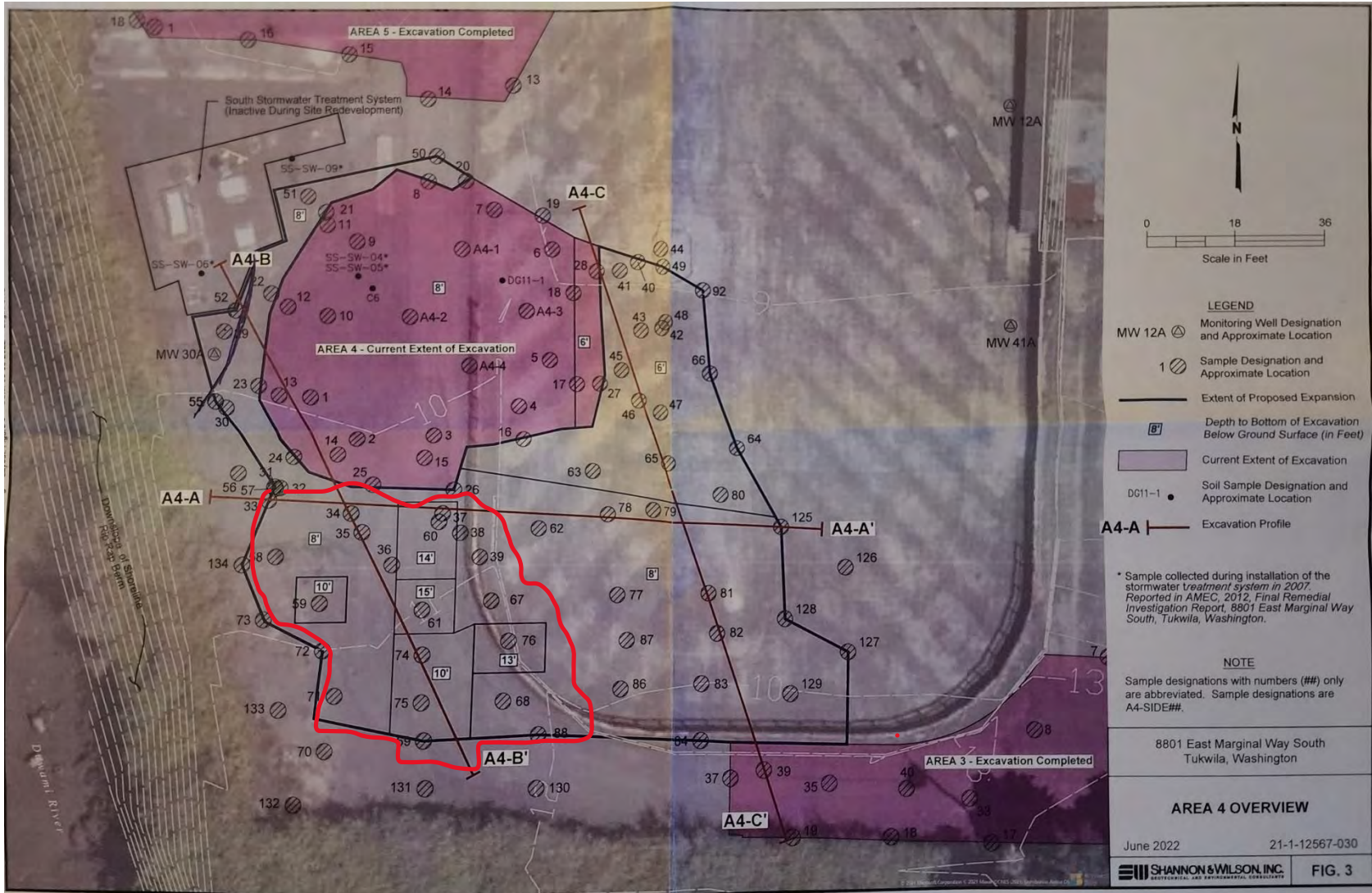
Figure 1. Map of planned excavation extent for PCB remediation. . Area circled in red is current extent of excavation as of 8/19/2022.
