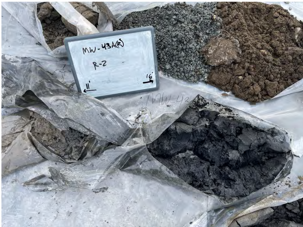
Figure 4: MW-43A(R) Soil Extraction 11-16 ft bgs
