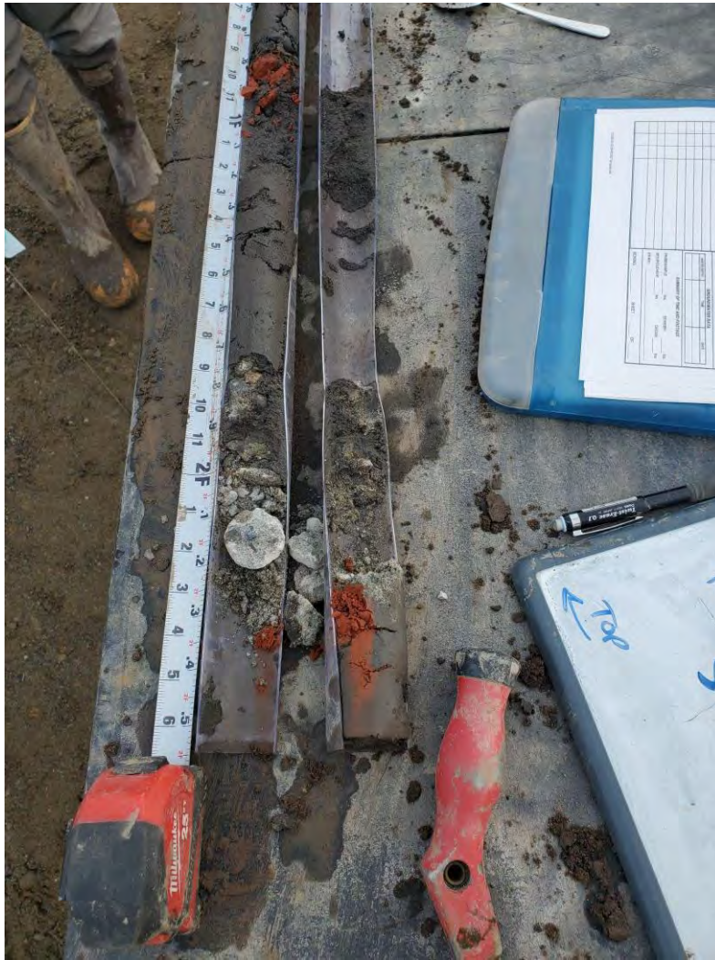
Figure 4. Brick and concrete found 5-10ft between area 4 and 5
