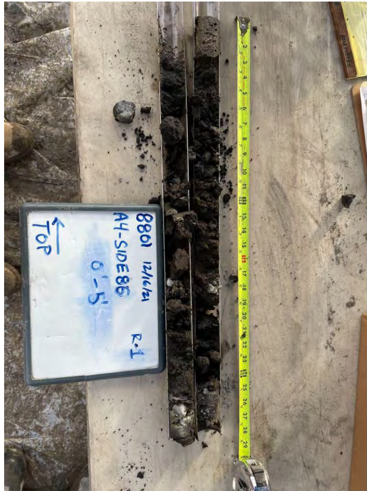
Figure 22. Area 4-Side 86: 0-5ft, 2:15pm (concrete at 5ft)
