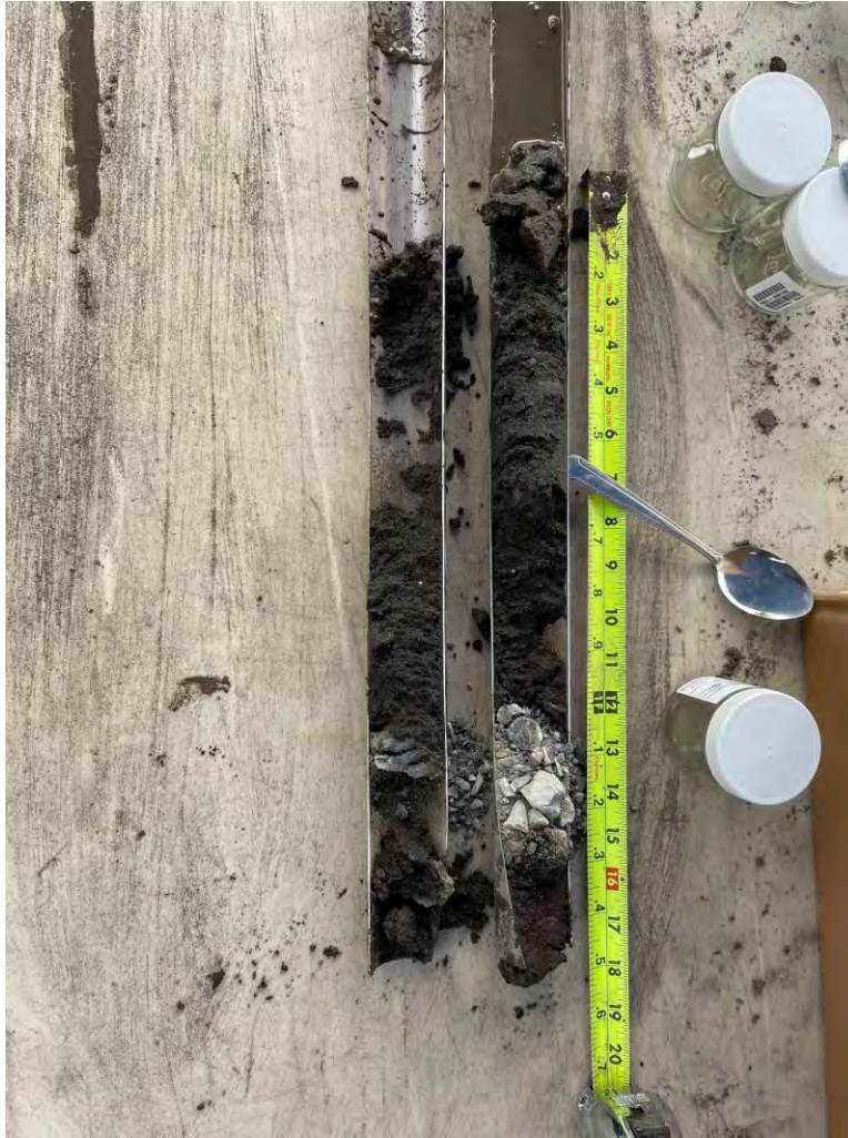
Figure 19. Area 4-Side 83: 3-6ft, 1:04pm (concrete at around 4-5ft)
