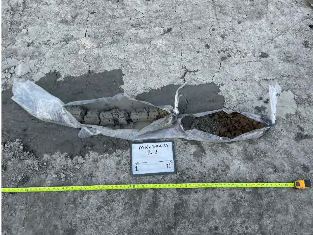
Figure 9: MW-30A(R) Soil Extraction 1-11 ft bgs
