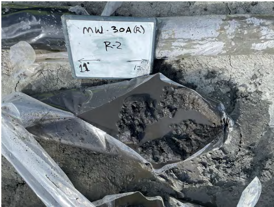
Figure 10: MW-30A(R) Soil Extraction 11-17 ft bgs
